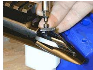
Secure the Bedding Block.
