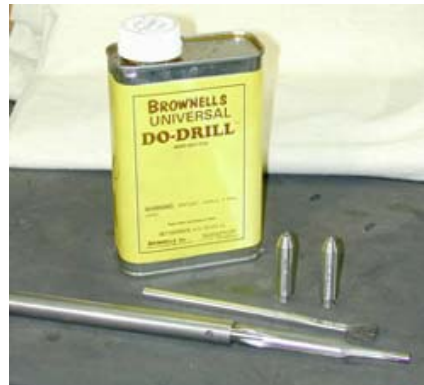
The tools for chambering. Do-Drill, GO and NO GO headspace gauges, a small brush for cleaning chips and the chambering reamer and extension.
