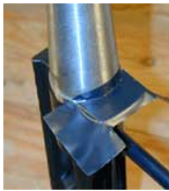
Stretch the vinyl tape across the lug and up the barrel.
