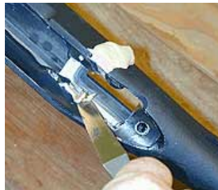
Start removing modeling clay, bedding tape and Compound that has oozed into various places.
