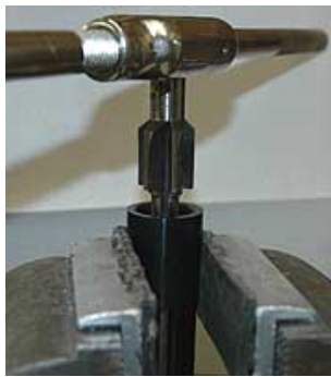
The Piloted Receiver Reamer ready to do its job
