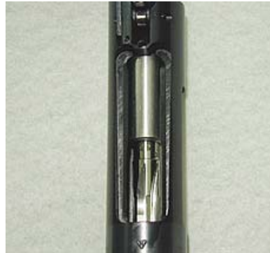
The reamer, with extension in place, started into the barrel.
