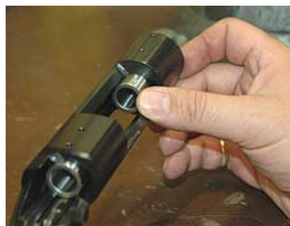
Slip the Manson Tooling Bushings into the action
