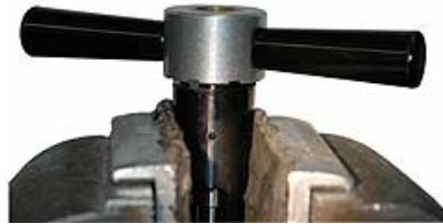
Receiver Ring Facing Tool in place on the shank of the Receiver Tap.
