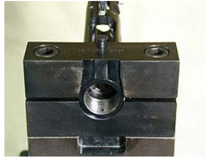
Our 700 Action in the Brownells Action Wrench. Note the screw in the wrench head to help locate the action correctly, and the cutout for the Recoil Lug.
