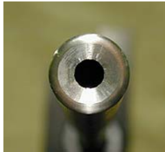
The finished muzzle crown and chamfer.
