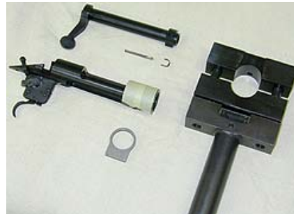
The taped action, the wrench with Remington 700 head attached, and the bolt, with firing pin, ejector and extractor removed.
