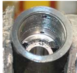
The lug face needs just a whisker more taken off to be completely faced.
