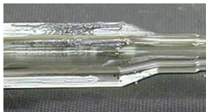
Early cuts will produce chips well back in the body area of the chamber.
