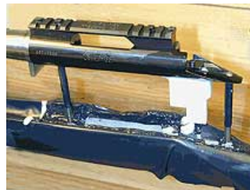
Dropping the barreled action into the stock.
