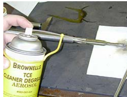
Clean the reamer and chamber thoroughly with TCE. Use a small brush to get rid of stubborn chips.
