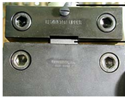
The action (top of photo) is almost completely screwed onto the barrel. The barrel is clamped in the Barrel Vise (lower edge of photo). The barrel lug (center of photo) covers the remaining exposed threads.
