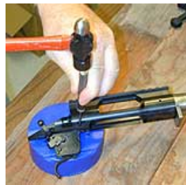
Driving out the front trigger group pin.
