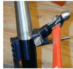
Tapping with the hammer will cut the tape cleanly.
