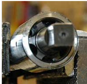
Our receiver face was definitely a bit crooked and needs only a couple of more revolutions of the Facing Tool to be dead-on square.
