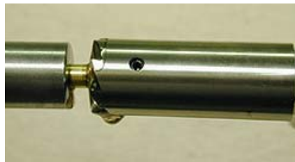
The 79° cutter in position to make the crowning cut.
