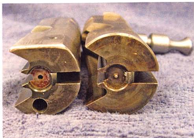
The original bolt (r.) shows the fixed firing pin typical of Stens. Matthews needed to replace this with a moving firing pin that would be driven forward by a hammer.
