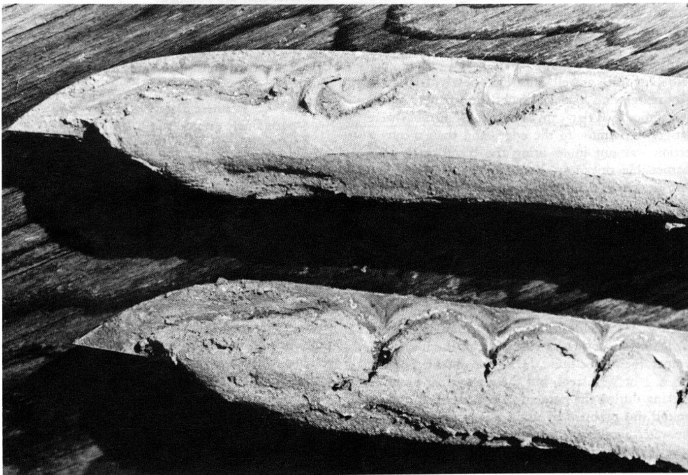
Fig. 156. Close-up of blade covered in the heat-treating clay
