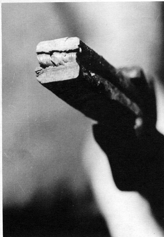
Fig. 119. End view of the fold. Note that laminations are visible on the chiseled surfaces.
