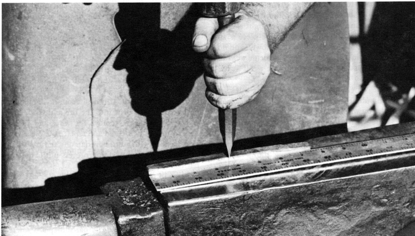
Fig. 117. Bar is chiseled three-quarters of the way through to aid in folding the bar in half.
