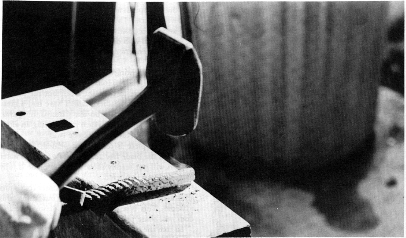
Fig. 144. Welding the cable into one piece
