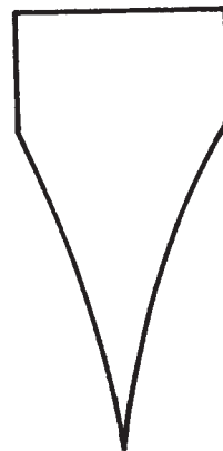
Fig. 39. Cross section of a hollow, or concave, ground blade.
