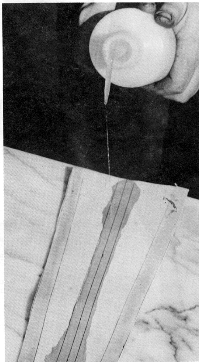
Fig. 82. Acetone is applied to the leather to make it moldable, but be careful to keep the acetone away from the cemented areas as such contact will remove the contact cement, making the cement useless.
