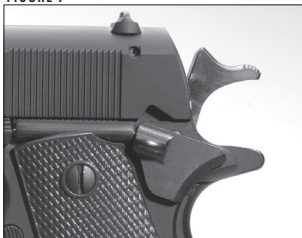
The hammer in the half-cock position.
