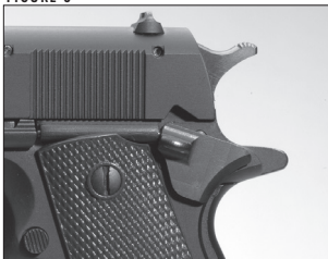
The hammer in the dropped position.
