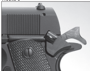
The hammer in the full-cock position.
