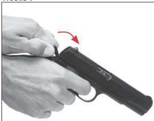
Lowering the hammer to the dropped position.
