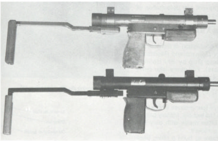
Improved prototype, including plugs without threading, welded bracket, and plastic pistol grip (top) compared with the standard prototype (bottom).
