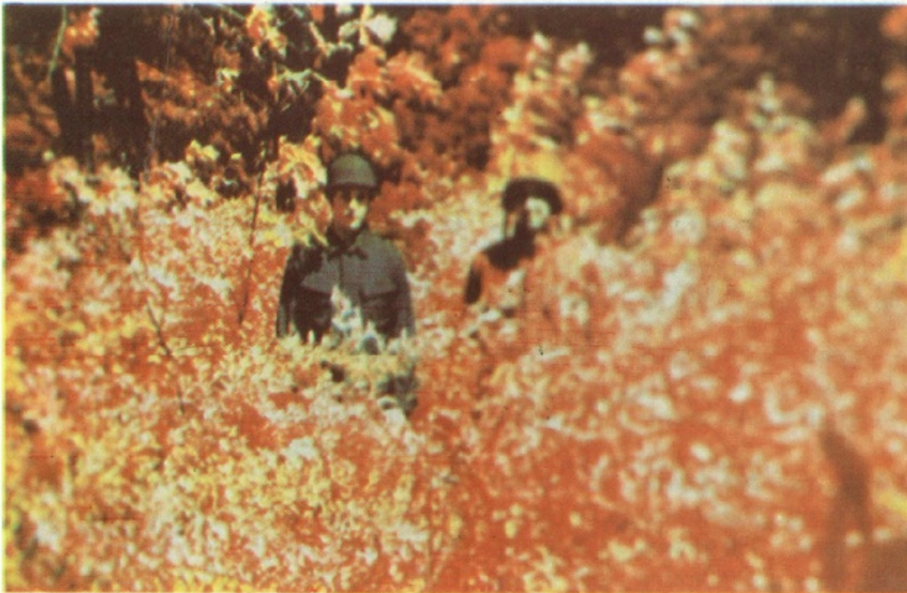
This infra-red photograph shows the effect of incorporating carbon into the camouflaged uniform material. Left: figure without carbon; Right: figure with 4% carbon.
