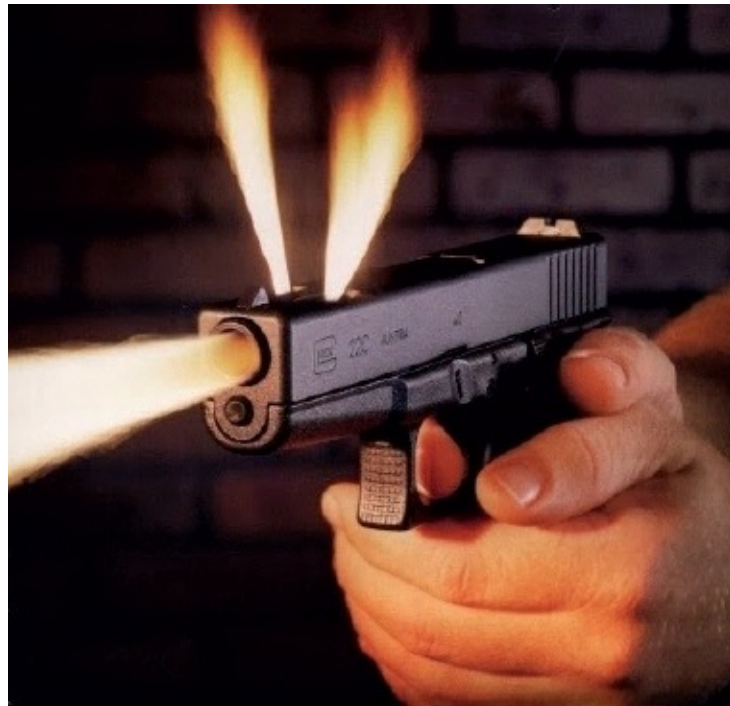
The G22C spits flames. The slots in the barrel and slide help a user control muzzle flip. Image courtesy of GLOCK, USA.
