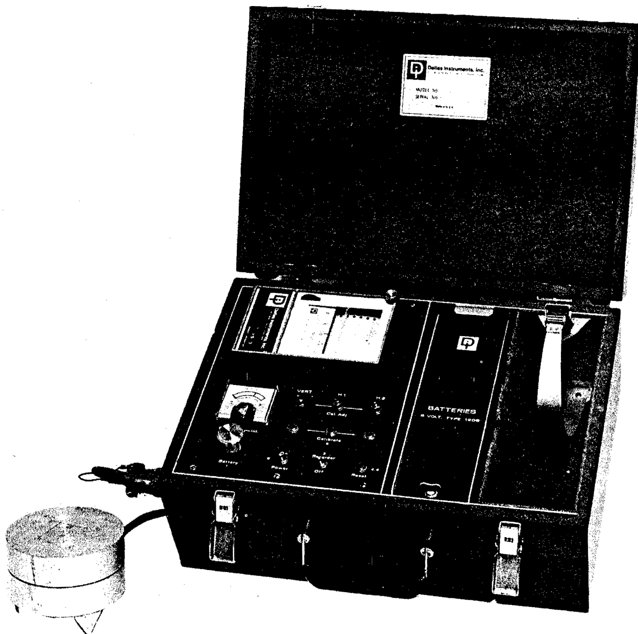
Figure 94.—Seismograph for measuring ground vibrations from blasting.
