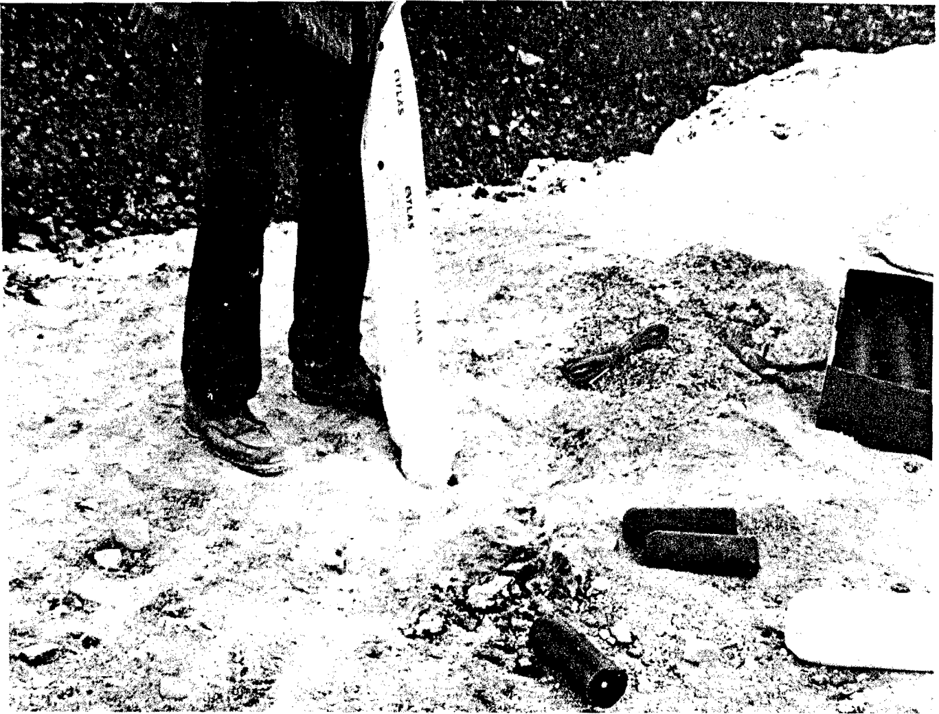
Figure 56.—Pouring slurry into small-diameter borehole. (Courtesy Atlas Powder Co.)
