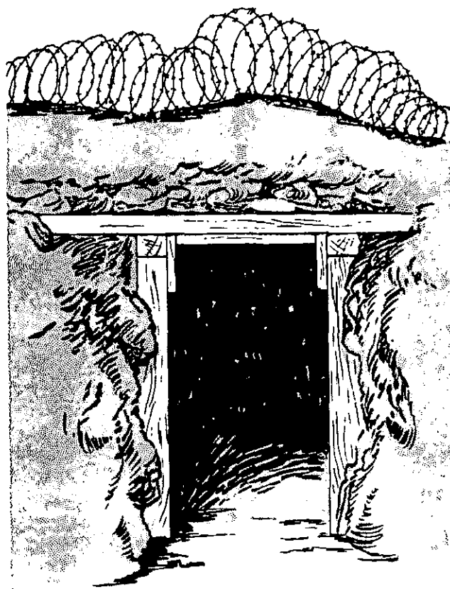
Figure 6-2. Protective wire on top of overhead cover.
