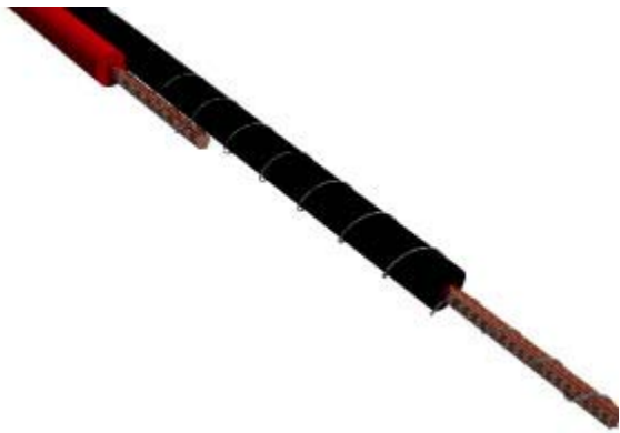
[Fig.1. Detail of method for wrapping Nichrome wire]
