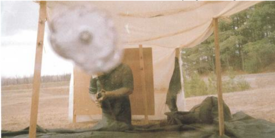
The resulting hole from a 7.62mm/.308-caliber round fired from a USMC M40 A1 sniper rifle during through-glass testing at Quantico.
