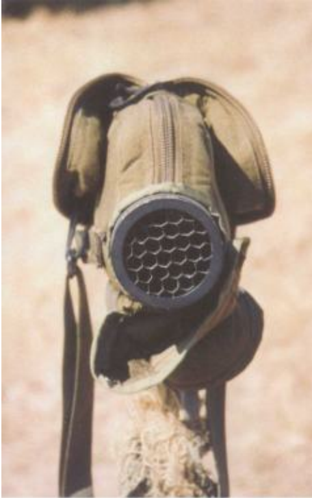
The Leopold x40 spotting telescope.. Note the honeycombed kill-flash lens cover designed to stop the sun's rays reflecting off the lens and compromising the sniper.
