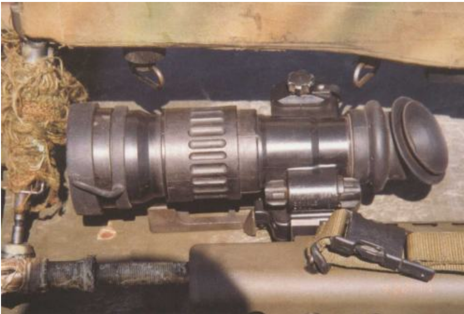
The Pilkington Kite sight, or Common Weapon Sight in British Army use. The CWS night sight works by gathering available light and amplifying it to produce an image. The commander with up to four snipers' views on a split screen, or a single sniper's view on a full screen. Full recording facilities are provided and the unit can also be linked via the Internet to authorized users anywhere in the world, using an on-line encryption system.
