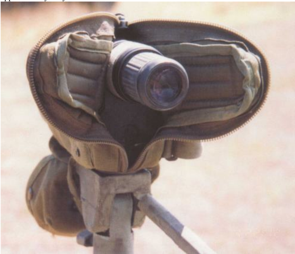
The Leopold x40 spotting scope comes with a padded cover that semi-camouflages as well as protects the scope, with easy-access zippered openings at the eye piece and a drop-down flap cover for the objective lens.
