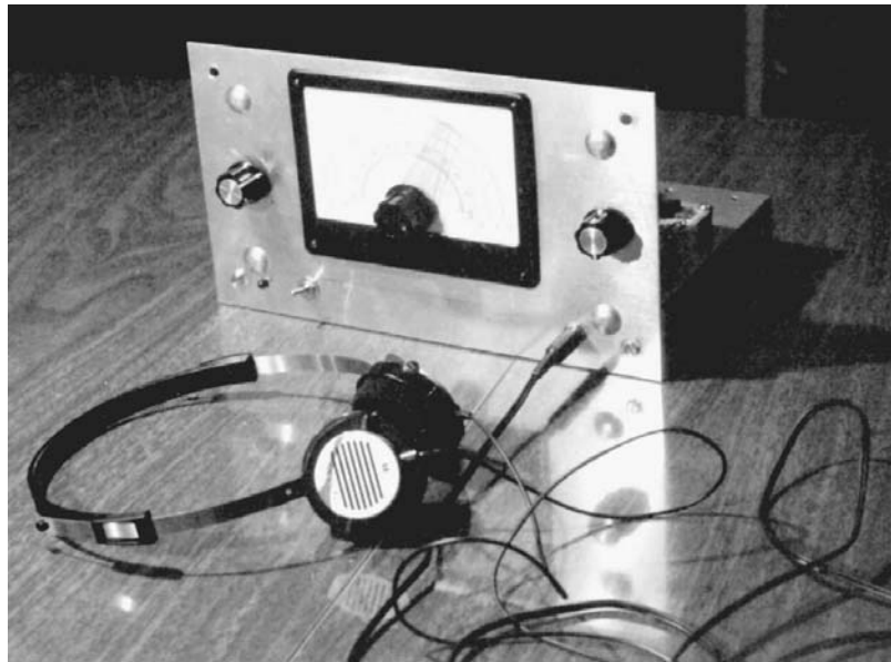
6-17 Photo of direct-conversion receiver.
