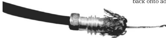
(C) Coax stripped and shield laid back onto adapter
