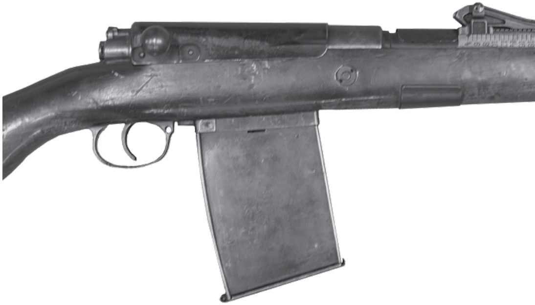
A Gew 98 fitted with a sheet-metal bolt protector and 20-round extension magazine. (Author's photograph, © Royal Armouries PR.6414)
