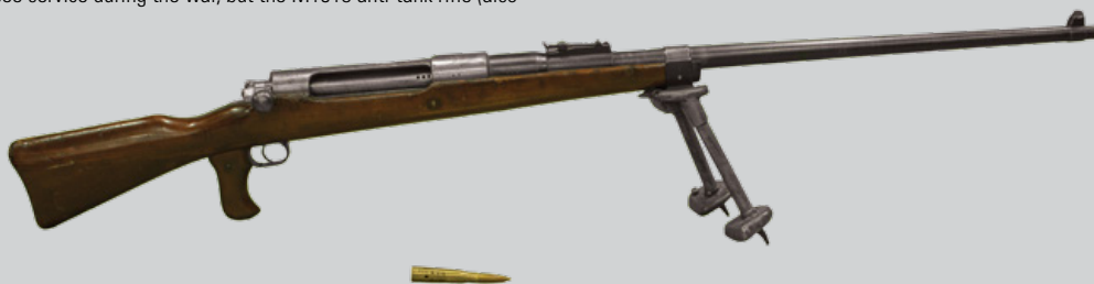
ABOVE The Mauser M1918 T-Gewehr and its 13.2×92mm cartridge. The three holes drilled in the cartridge and bolt are to deactivate the weapon, not original features. (Author's photograph, © Royal Armouries PR.1725)
