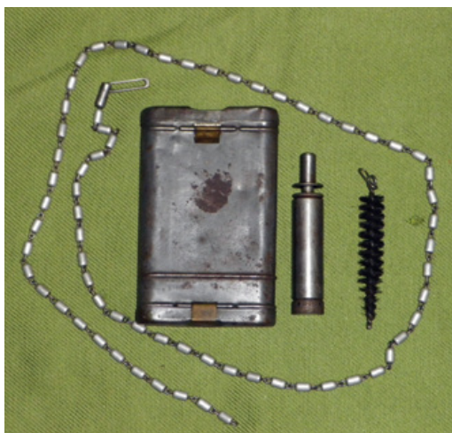
The Reiningungsgerät 34 cleaning kit, with chain pull-through, oil bottle and chamber brush. Unfortunately, the bore brush and take-down tool are missing from this example. The kits were originally well made, but quality declined through the war years. (Author)
