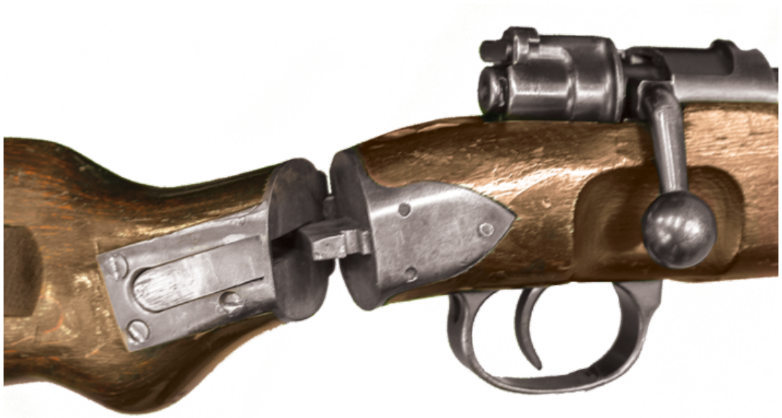
The hinge of the folding stock of the prototype paratrooper version of the Kar 98k. (Author's photograph, © Royal Armouries PR.6441)
