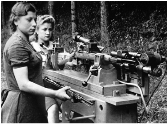
Two female workers posing with a 'shooting machine' used to test sight alignment, probably at the Mauser factory at Oberndorf. The joint Mauser/Zeiss machine allowed a task that had previously required a trained marksman to be done by unskilled workers, provided they followed the steps correctly. The author is not able to explain why the machine appears to have been set up outdoors. (Tom Laemlein/Armor Plate Press)
