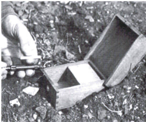
The small size of the German Schü-Mine 42 is apparent here; fitting a large charge to antipersonnel mines was simply wasteful, since just enough to blow off a foot would at once take three men out of the line – the casualty himself, plus two others to carry him. Here the GI's hand holds the removed Z.Z. 42 pressure fuze (dark color) and detonator, and the 200g charge is seen in the wooden box. The fuze had a Bakelite® body and only the striker and tripwire loop were steel, so it would not register when ground was being searched with an electronic/magnetic mine detector.
