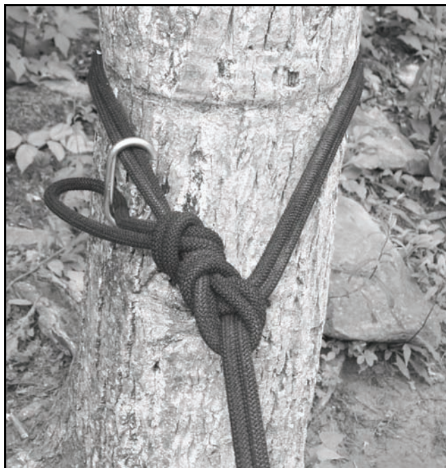
Figure 2-1. Rope tied to anchor with anchor knot.
