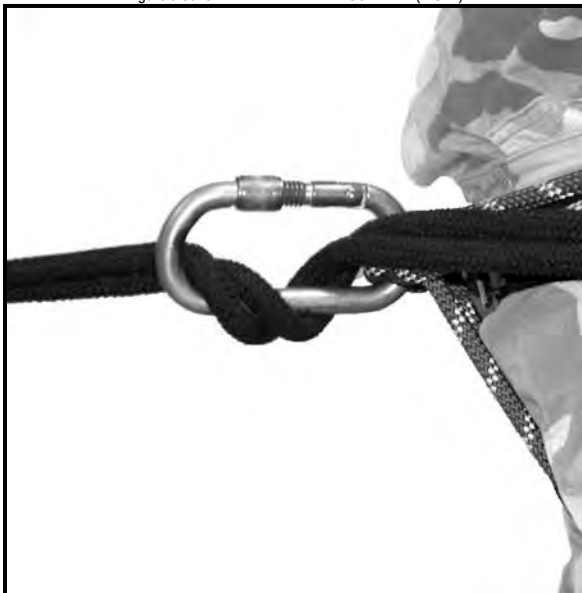
Figure 9-30. CARABINER WRAP DESCENDER (INSET)
