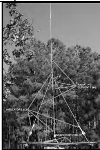
Figure 4-5. COMPLETED 292-TYPE ANTENNA
