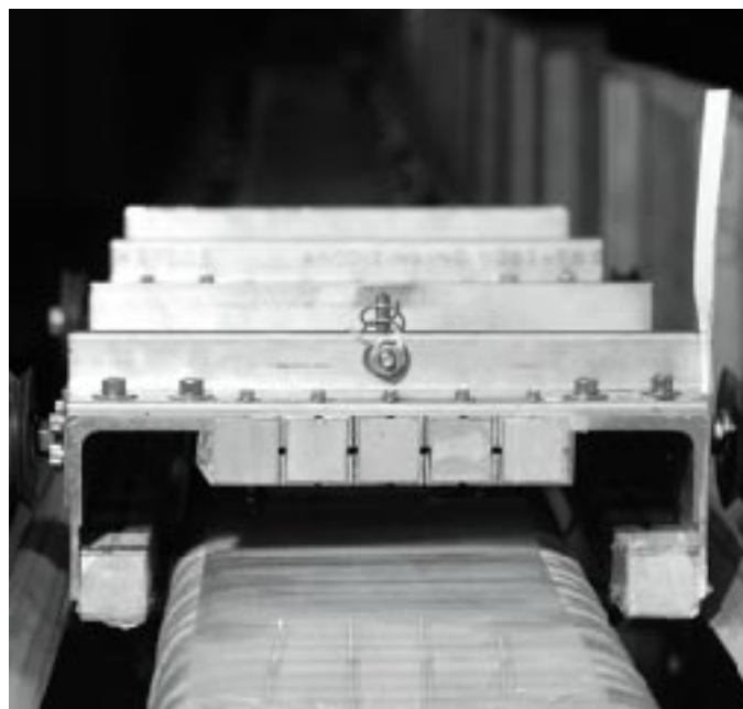
Figure 2. The test cart in motion levitated above the test track. The Halbach arrays can be seen beneath the cart and suspended from its sides. These arrays generate a magnetic field that induces, from the motion of the car, currents in the coils contained in the track, lifting and centering the cart above the track.
