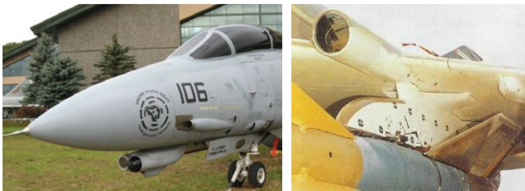
FIGURE 9. AN/ASX-1 TISEO IN PLACE ON F-14D NOSE AND F-4E WING 30
