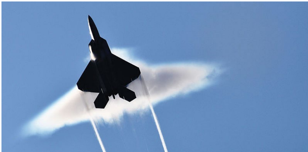
FIGURE 18. USAF F-22 WITH MACH CONE
