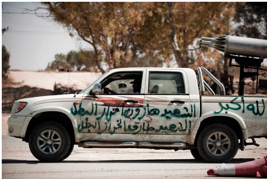
A Libyan militia Toyota Hilux mounting a 57mm UB-16-57 aircraft rocket pod in Misrata, 2011. Rebel slogans have been spray-painted over the side of the vehicle – a common affectation alongside the more usual decals and flags. (Photo by Gianluigi Guercia/AFP/Getty Images)
