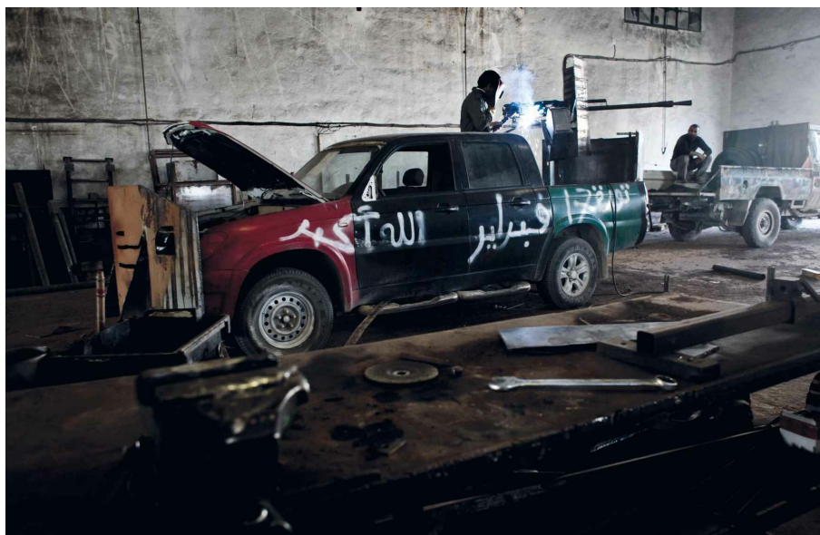
Inside a Libyan technical workshop where a welder works on mounting a 14.5mm KPV HMG behind a makeshift armoured gun shield in 2011. These workshops were responsible for many of the both innovative and crazy designs seen during the uprising against the regime and the later Libyan Civil War. (Photo by Etienne De Malglaive/Getty Images)
