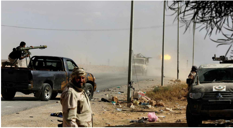
Pro-regime forces battle NATO-backed militias in 2012 from a number of Mitsubishi- and Zhongxing-based technicals. To the left is what appears to be a 73mm SPG-9 recoilless rifle, to the right a 12.7mm DShK HMG and in the background an unidentified 'heavy technical' fires what is likely a twin-barrel 14.5mm ZPU-2 cannon. (Photo by Mahmud Turkia/AFP/Getty Images)
