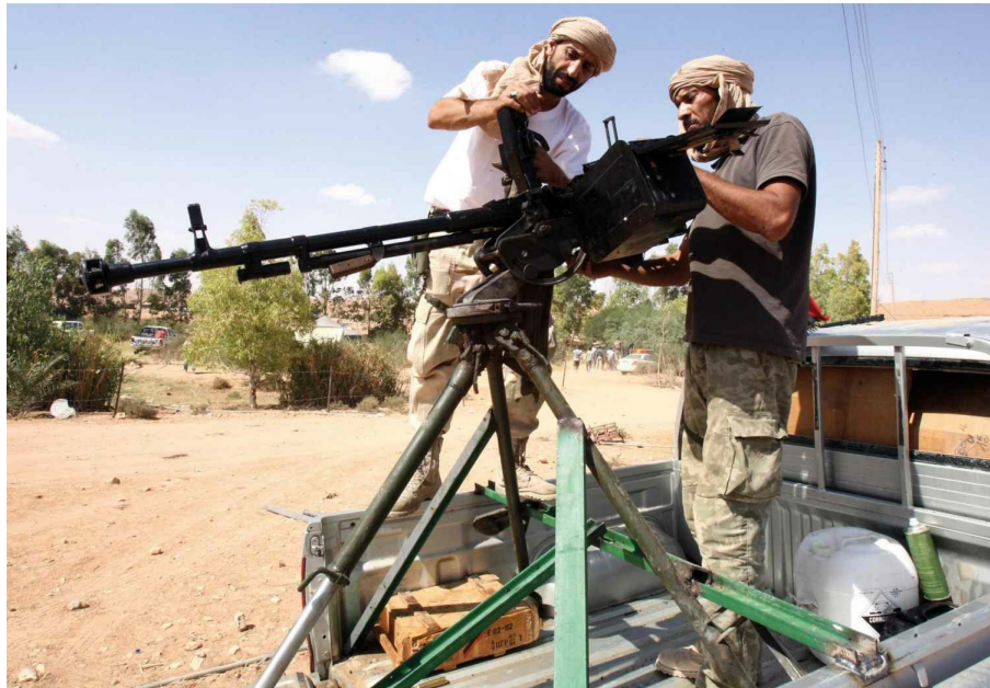
An excellent view of the types of mounts seen on Libyan technicals. This remarkably well maintained 12.7mm DShK HMG is affixed to a standard anti-aircraft tripod which is then held in place by crude brackets. Typically, it is missing its specialist anti-aircraft sight. (Photo by Mahmud Turkia/AFP/Getty Images)
