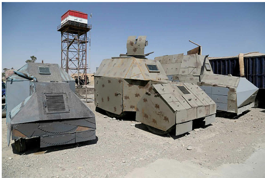
Homemade Islamic State armoured technicals built on a commercial light truck chassis designed as suicide vehicle-borne IEDs (SVBIEDs). Note the gun shields fitted to the centre vehicle which typically mounts a PK-series medium machine gun to suppress defenders as the car bomb is driven at the target. Such vehicles were much in evidence during the 2017 battle for Mosul and in Syria targeting Kurdish forces. (Photo by Yunus Keles/Anadolu Agency/Getty Images)
