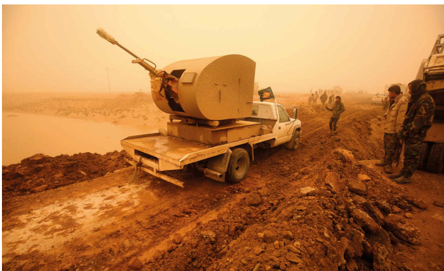
Pro-government Shia paramilitaries from the Popular Mobilisation Units (PMU) mounting a 23mm ZU-23-2 in a custom-made armoured turret, west of the Iraqi city of Mosul in 2016. The same turret has been mounted on heavily
