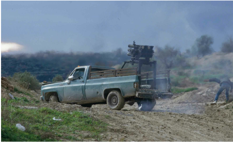
A 107mm Chinese Type 63 MLRS firing from a Dodge technical, Beirut, 1986, one of the earliest examples of a technical-mounted MLRS. Due to their inaccuracy, they are more of a terror weapon. (Photo by Maher Attar/Sygma via Getty Images)
