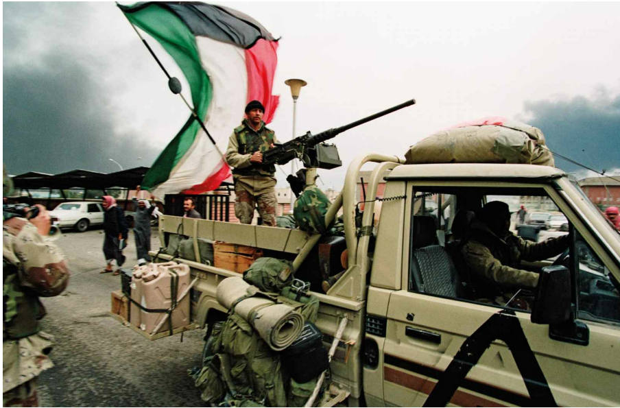
Members of the US Army's 5th Special Forces Group entering Kuwait City during Operation Desert Storm , 1991. These commercial FJ-series Land Cruisers were fitted with stowage racks and pedestal mounts for both .50 M2 HMGs and 40mm Mk19 AGLs, stencilled 'V' identification-friend-or-foe markings on the doors and bright orange VS-17 vinyl panels on the roof to identify them to Coalition aircraft overhead. (Photo by Jacques Langevin/Sygma/Sygma via Getty Images)
