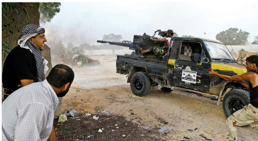
Anti-regime Libyan National Transitional Council (NTC) militia firing a Land Cruiser -mounted 23mm ZU-23-2 anti-aircraft cannon in Sirte, Libya in 2011. Note the NTC seal displayed on the door and the insurgent enthusiastically adding the fire of his Kalashnikov pattern assault rifle. The ZU-23-2 was the NTC’s primary direct fire ‘light artillery’. (Photo by John Cantlie/Getty Images)
