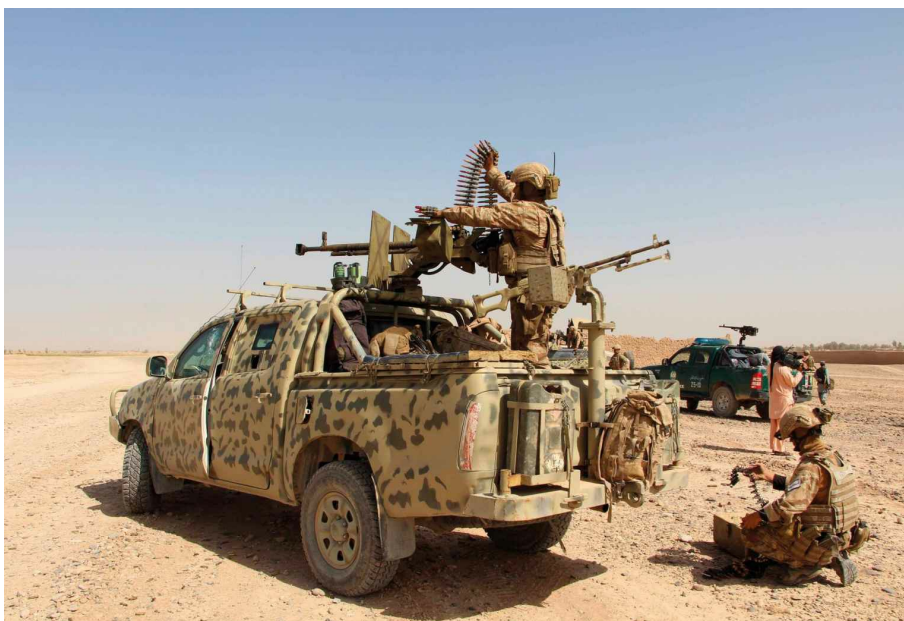
An Afghan National Army SOF technical mounting both 12.7mm DShK HMG and 7.62mm PKM MMG in Helmand Province, 2016. The Ford Ranger in the background belongs to the Afghan National Police and is likely also equipped with an older 7.62mm SG-43 MMG. The NATO-provided Rangers replaced a range of older model Toyotas. (Photo by Noor Mohammad/AFP/Getty Images)
