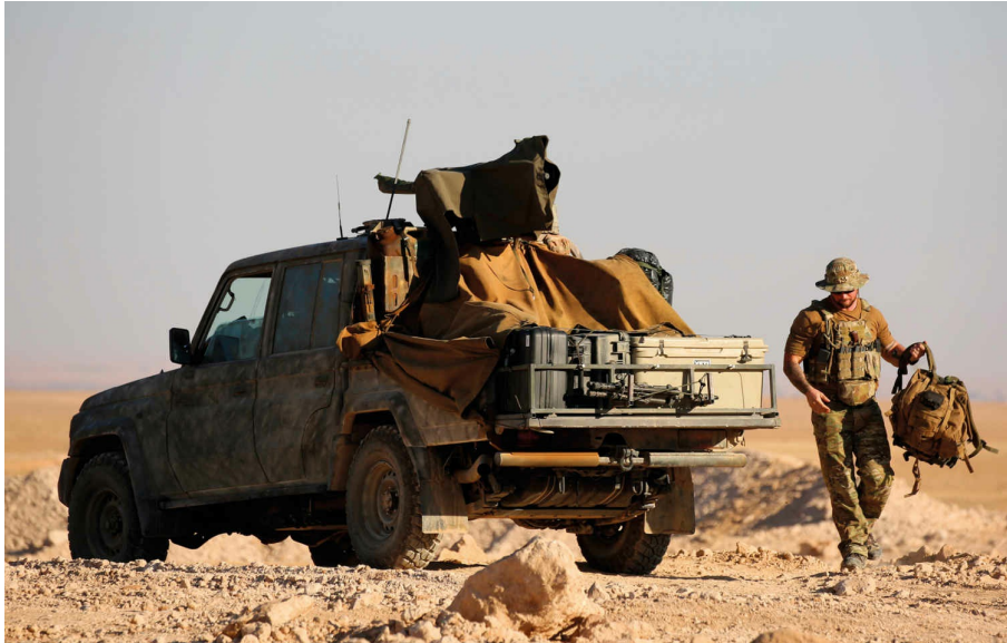
A Toyota Land Cruiser ‘Non-Tac’, photographed north of the Islamic State capital of Raqqa, being operated by unidentified US SOF in November 2016. The vehicle likely mounts a 40mm Mk47 Stryker AGL under the protective tarp. The Pelican cases carried in the stowage racks are for sensitive or fragile items like sniper rifles, cameras and optics. (Photo by Delil Souleiman/AFP/Getty Images)
