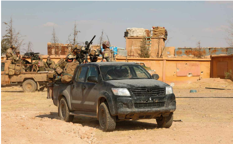
A Toyota Hilux operated by unidentified US SOF, possibly a Green Beret ODA (Operational Detachment Alpha), outside Raqqa, May 2016. The Hilux looks remarkably unaltered apart from the satellite communications (SATCOM) antennae on the roof and the pedestal mount .50 M2 QCB HMG which appears to mount the SureFire HellFighter Heavy Gun Spotlight offering both infrared and white light and an EOTech Holographic Weapon Sight. In the background is another SOF vehicle – which appears to carry US Navy SEALs again, based on the uniforms and plate carriers worn – equipped with a 40mm Mk47 AGL. (Photo by Delil Souleiman/AFP/Getty Images)
