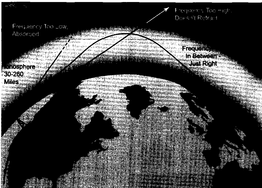
Figure 4-3 — Signals that are too low in frequency are absorbed by the ionosphere and lost. Signals that are too high in frequency pass through the ionosphere and are also lost. Signals in the right range of frequencies are refracted back toward the Earth and are received hundreds or thousands of miles away.
