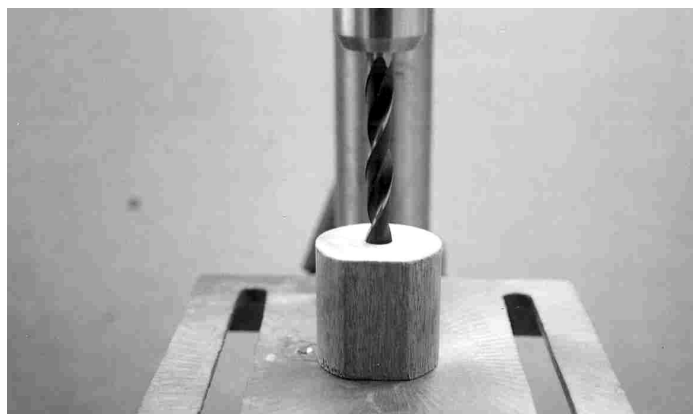
Drilling the bores.
