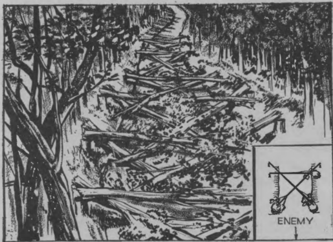
FIGURE 111.—Abatis constructed of interlaced trees in defile.
