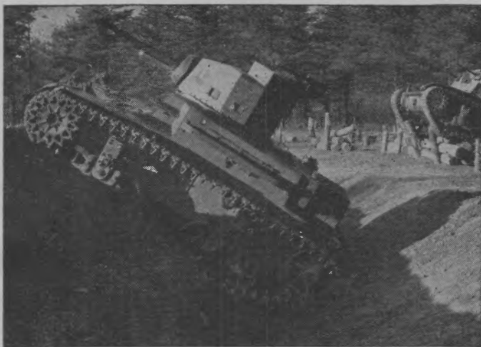
FIGURE 109.—Tank stopped by antitank ditch.
