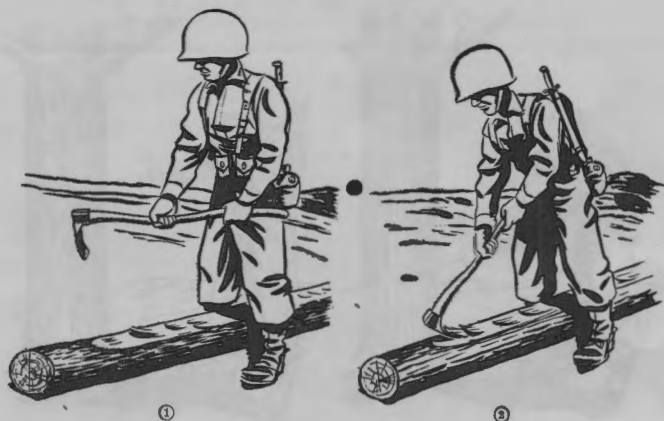
FIGURE 5.—Using the adz.
