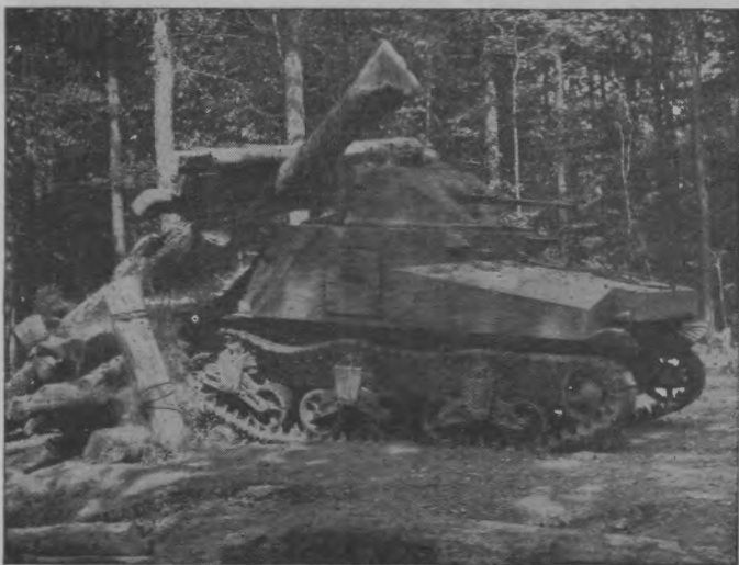
FIGURE 110.—Tank stopped by log wall.
