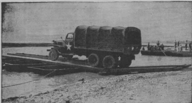
FIGURE 127.—Loading the raft.
