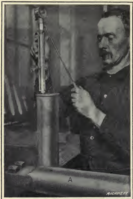
Fig. 179. Testing Hardness of Cartridge Cases with Scleroscope
