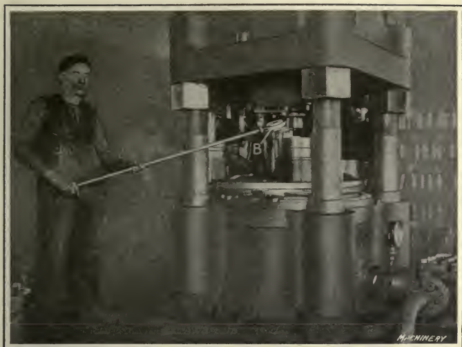
Fig. 174. Heading Cartridge Cases on a C. P. R. Heading Machine
