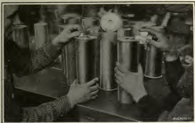
Fig. 159. Gaging Thickness of Flange and Thickness through Primer Hole
