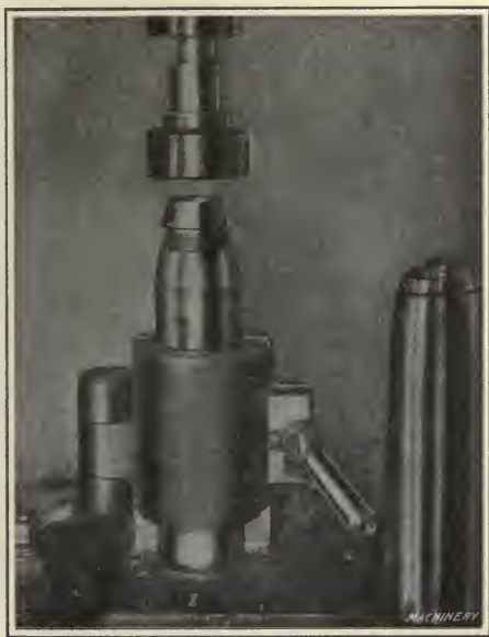
Fig. 61. Assembling Ogive In Shell Nose
