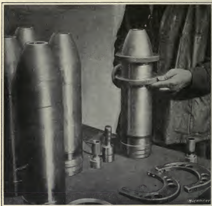
Fig. 89. Gaging External Diameter and Thread In Nose
