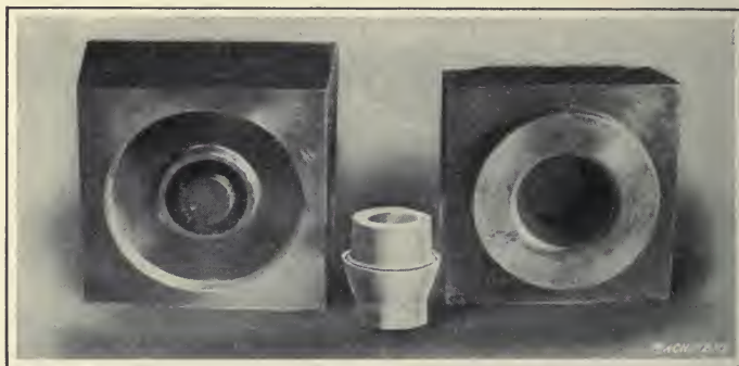
Fig. 131. Upper and Lower Dies used in Press shown in Fig. 129.
