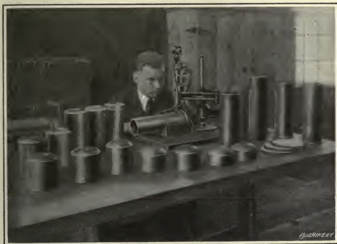
Fig. 163. Testing Hardness of Cartridge Case with Scleroscope
