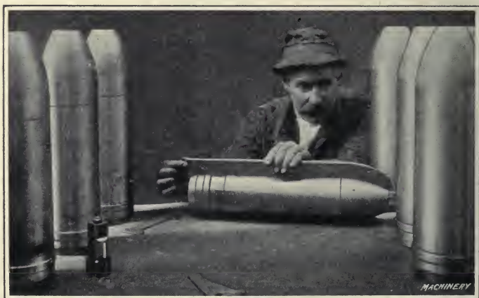
Fig. 90. Gaging Contour of French 120-millimeter High-explosive Shell
