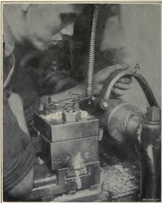
Fig. 74. Facing off Closed End of Forging to Length
