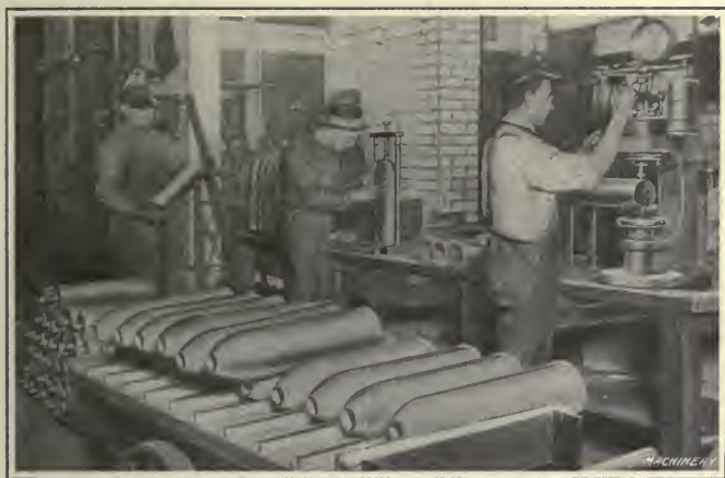
Fig. 81. Testing Hardness of French 120-millimeter High-explosive Shells
