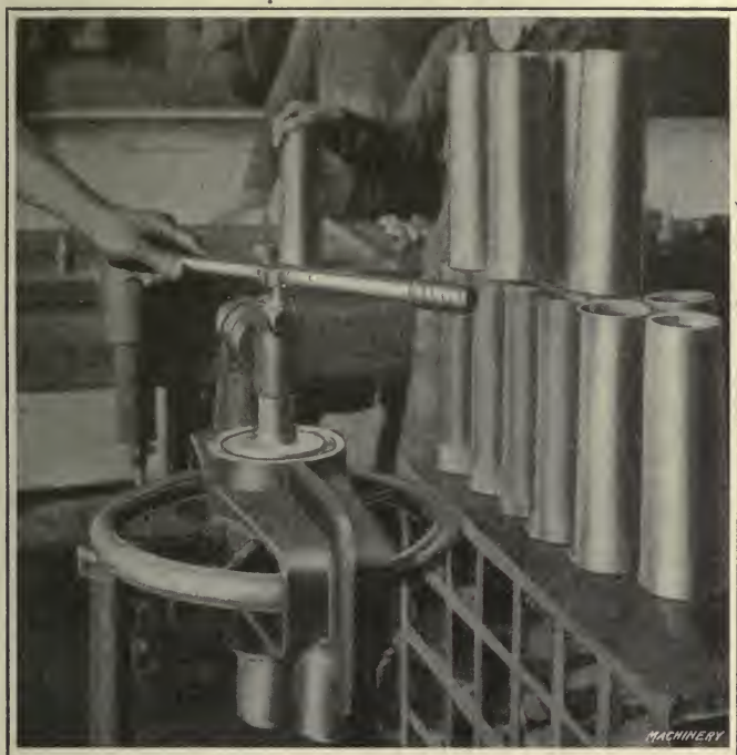
Fig. 178. Hand-reaming Primer Pocket In Head of Cartridge Case
