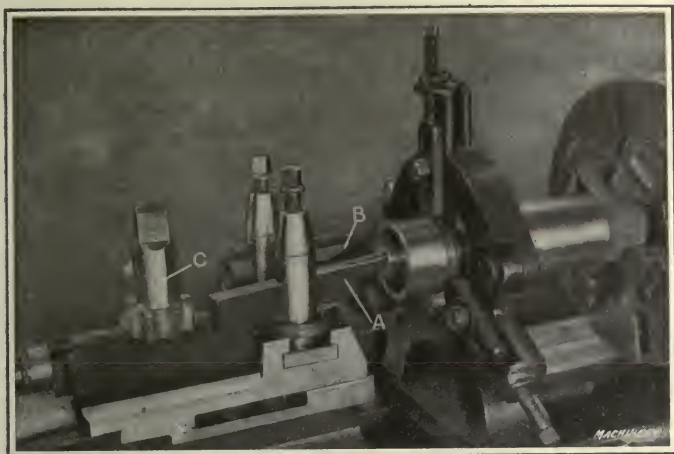
Fig. 53. Facing and threading Nose of High-explosive Shell
