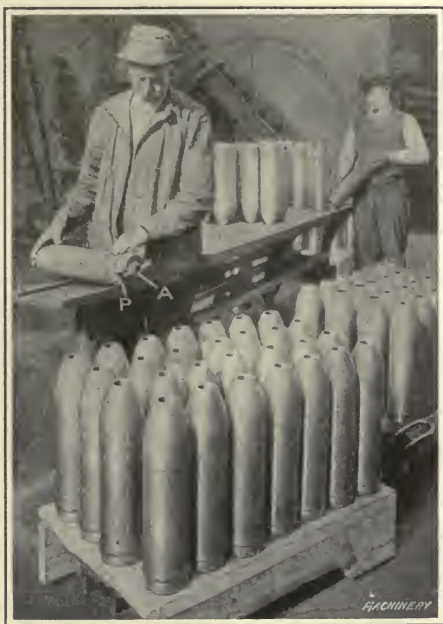
Fig. 93. Gaging Concentricity of Shell
