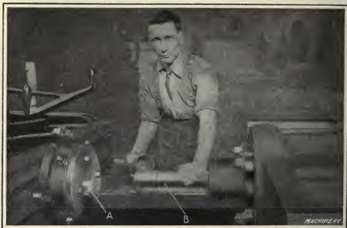
Fig. 172. Third Redrawing Operation on Williams & White Bulldozer
