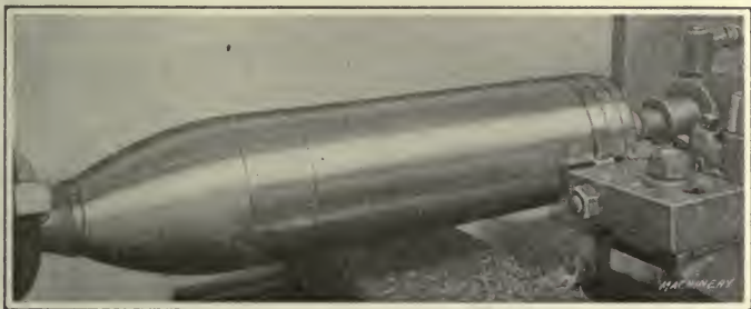
Fig. 87. Turning Copper Driving Band
