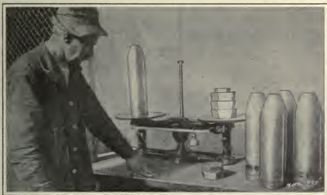
Fig. 88. Weighing French 120-millimeter High-explosive Shell
