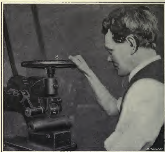
Fig. 38. Stamping in a Holden-Morgan Rotary Stamping Machine
