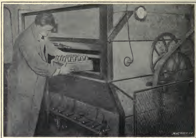
Fig. 137. Baking Varnish on High-explosive Shell Fuses
