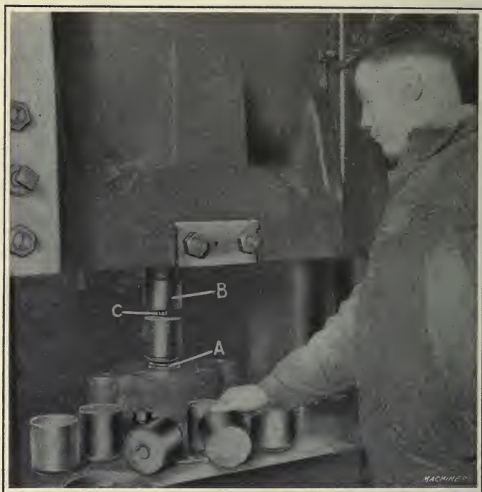
Fig. 146. First Indent on a Toledo Press
