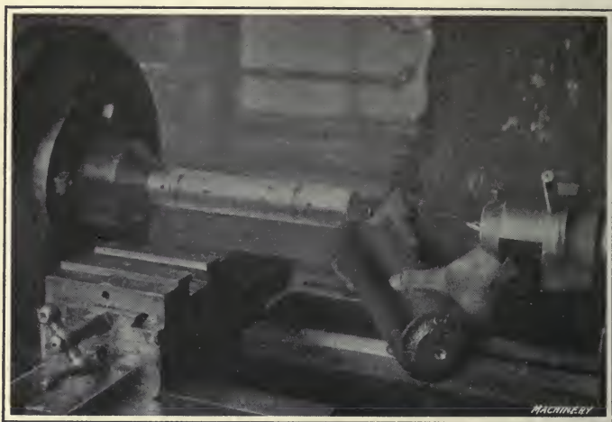
Fig. 58. Centering Closed End of Forging
