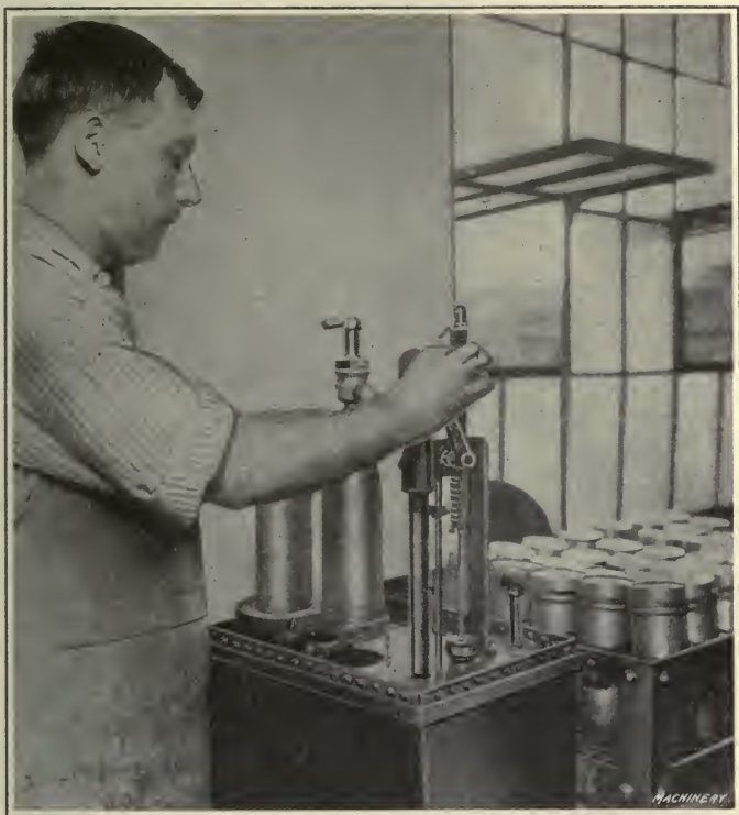
Fig. 37. Varnishing Interior of High-explosive Shells
