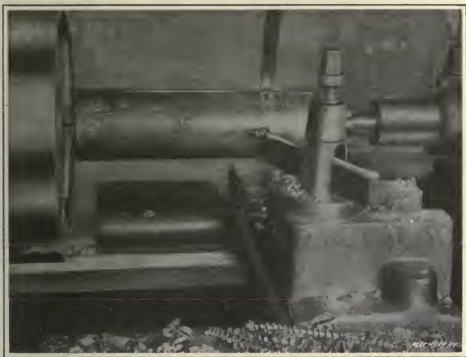
Fig. 59. Rough-turning External Diameter of Shell
