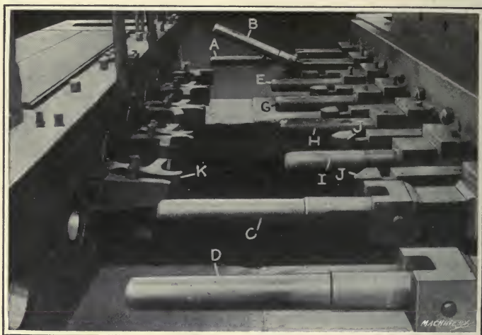
Fig. 23. Arrangement of Dies and Punches on Williams & White Bulldozer for forging Russian High-explosive Shells
