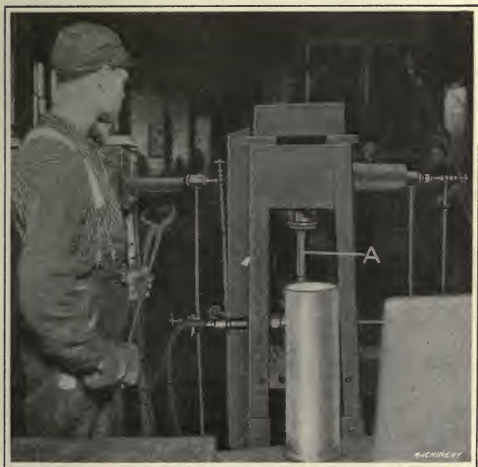
Fig. 175. Mouth-annealing Cartridge Case In an Improved Annealing Furnace
