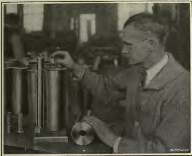
Fig. 156. Gaging Thickness of Head of Cartridge Case
