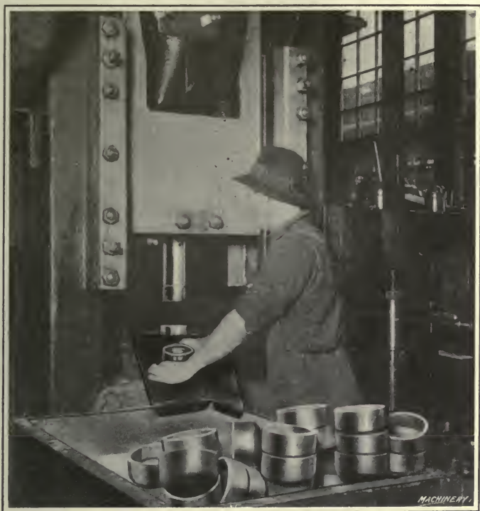
Fig. 145. First Redrawing Operation performed on a Toledo No. 59 Press
