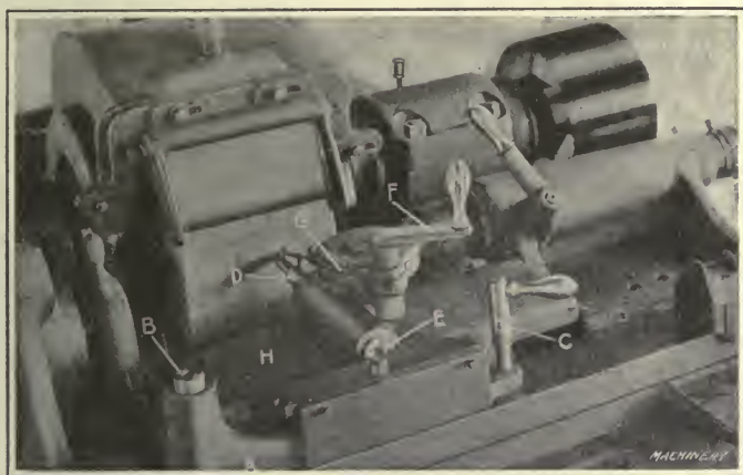
Fig. 121. Wheel-truing Device used on Ford-Smith Grinding Machine
