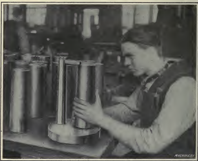
Fig. 158. Gaging Over-all Length of Case
