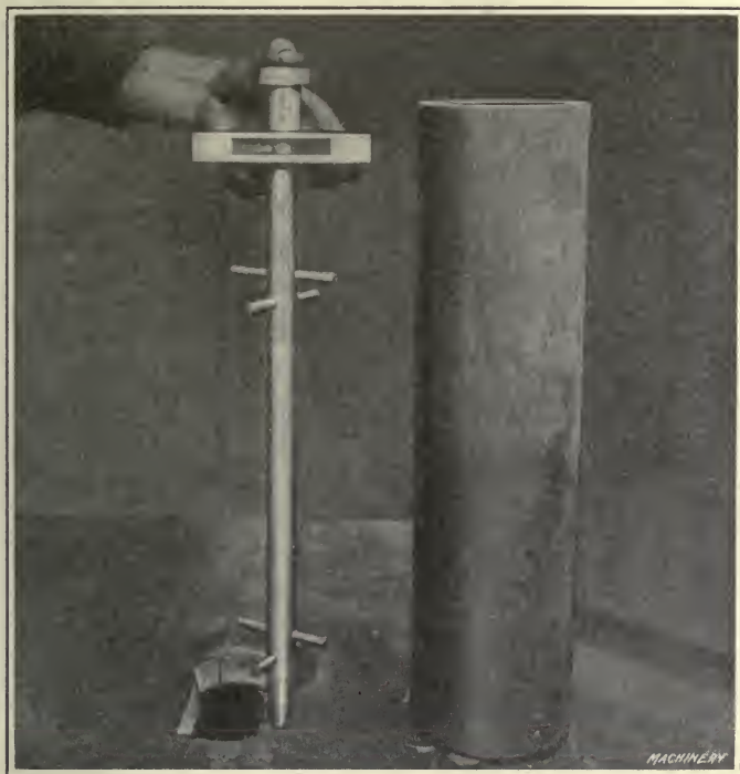
Fig. 71. Gage used in testing Length of Trimmed Forgings
