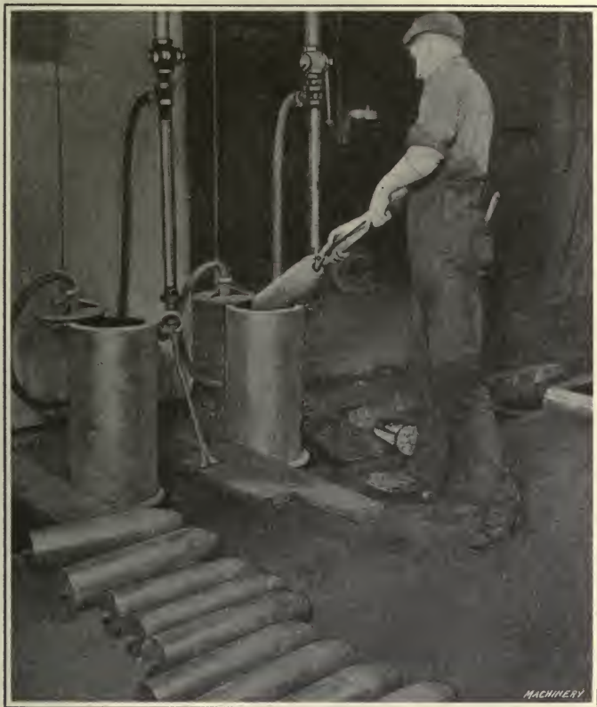
Fig. 79. Dipping French High-explosive Shells in Special Cooling Bath
