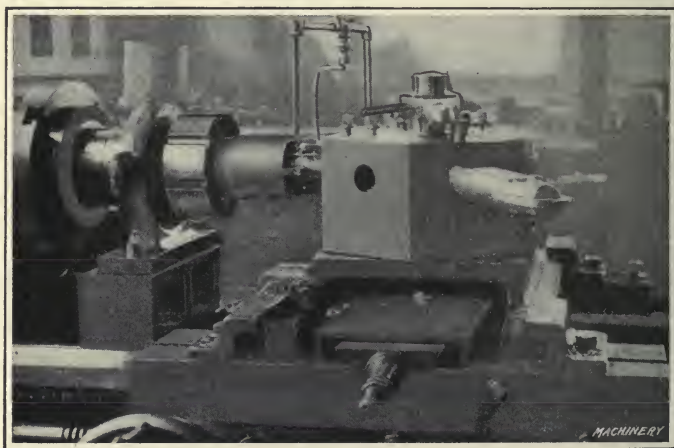
Fig. 97. Finish-boring, reaming and facing 4.5-Inch Howitzer High-explosive Shell
