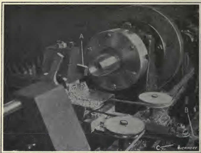
Fig. 62. Turning Ogive in Open End of Shell
