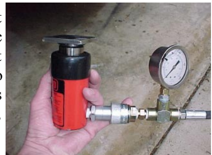
Closeup of cylinder & gauge.
