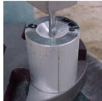
Arbor press pin pre-pressing tracer compound
