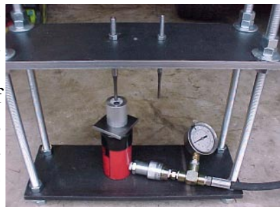
Press frame with cylinder & bullet die on cylinder
