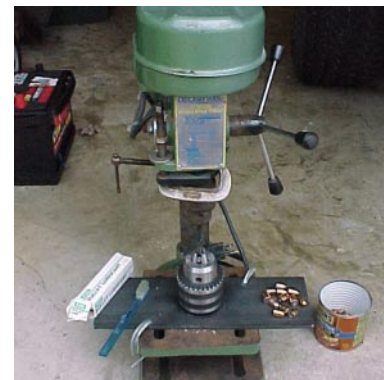
Note C-clamps holding chuck/plate to drill press table.
