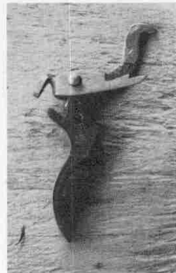
Trigger with trigger bar pinned in place.
