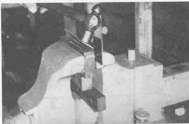
The flange, which will form the lower side, is folded 90 degrees with a heavy hammer.
