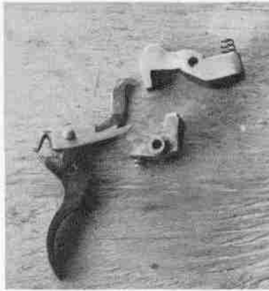
Component parts of trigger assembly.
