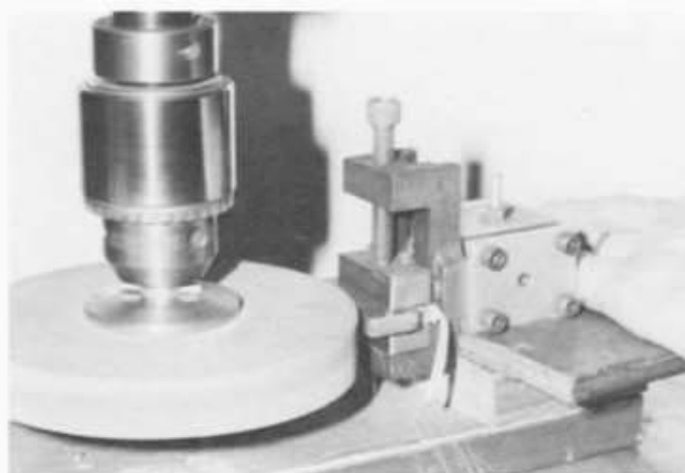
Fig. 5-18 This shows the drillpress set-up to grind the support shoulders. See text for further details.
