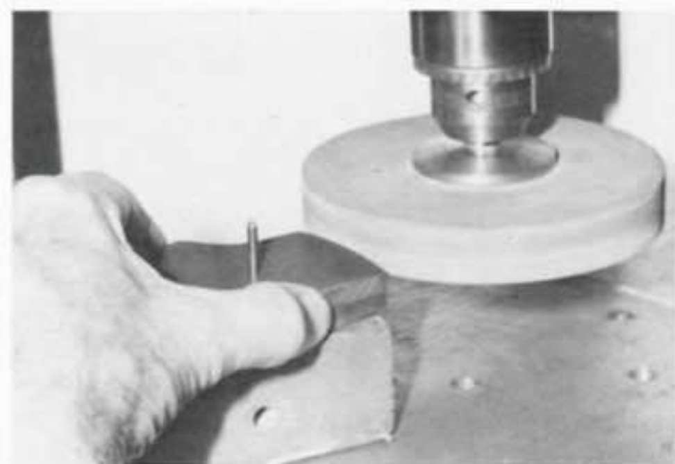
Fig. 5-17 As described in the text, this photo shows the drillpress set-up to grind the radius surface on the rear of the breech block sides.
