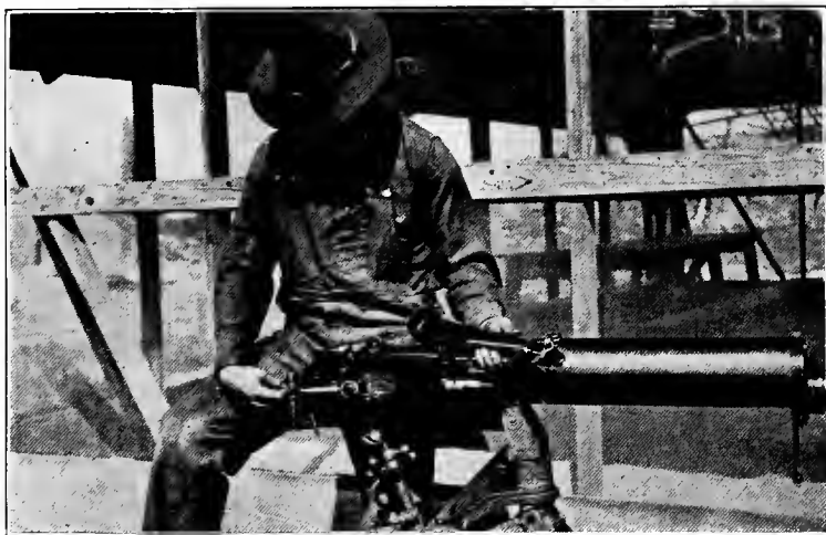
Testing friction of recoiling parts. Note position of roller handle, also that recoil spring is removed during this test.
