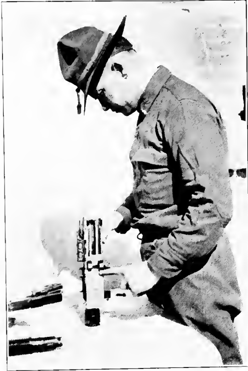
Examination of receiver to see if thin part of bottom plate at point indicated has been dented in
