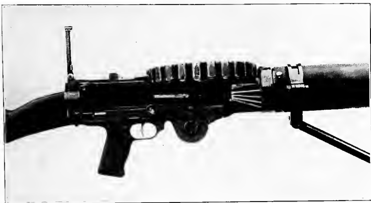
Second characteristic position of charging handle
