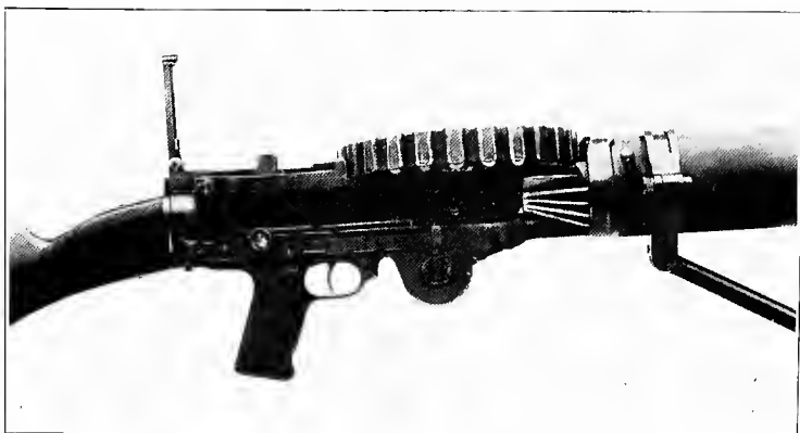
Fourth characteristic position of the charging handle
