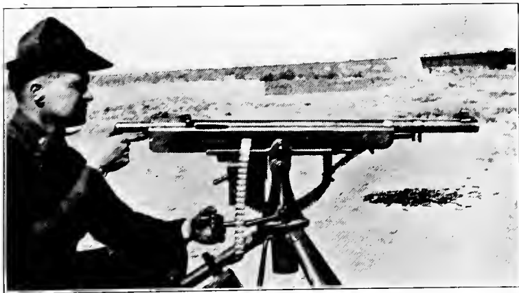
Third characteristic position of gas lever. Note that gas lever is all the way back.
