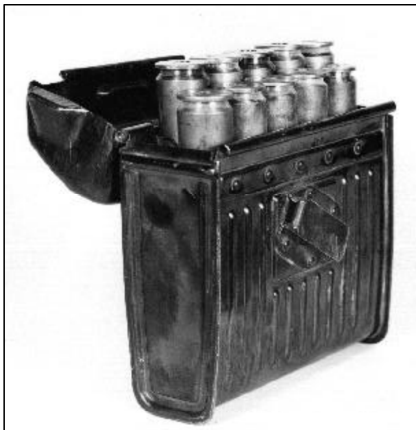
A metal ammunition carrier could be mounted on the sides of the P.z.B. anti-tank gun for easy access by the operator of the weapon. Each carrier held 10 rounds of ammunition. (NARA photo)
