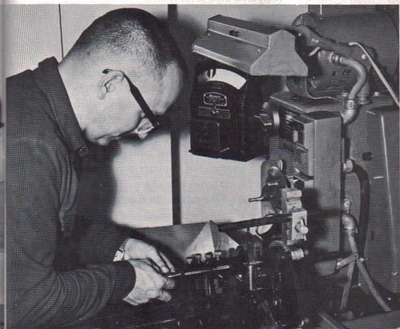
Rorschach, left photo, hones the "bores" of core-forming and core-seating dies to within 50 millionths of an inch of final size in a series of operations, then takes the last .00005 with a wood lap and 60,000
