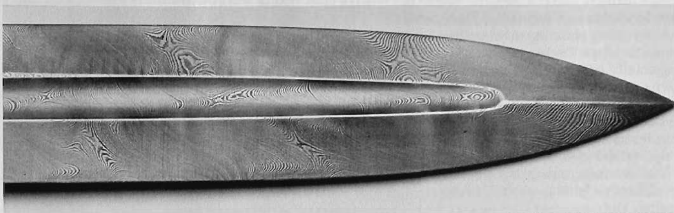
A maiden's hair pattern made by the author. This is another more commonly seen design. The patterning can be bold or subtle, depending upon the materials used and the amount of layering. Materials are 1095 and meteoric iron. (Photo by Gary Thompson)
