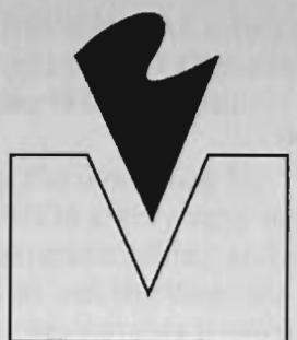
WELDED/TWISTED CORE CUT THREE- QUARTERS THROUGH WITH CHISEL.
