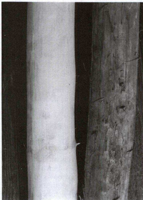
The white wood at left was cut in the summer, when pulling off the bark also removed the inner bark. The wood at right was cut in the winter, when the inner bark sticks tight to the wood.
