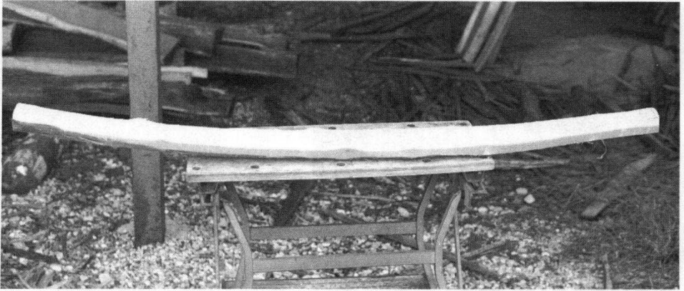
Sometimes wood from a small tree, and Osage in particular, will take a backset upon drying. This piece was flat when first split.
