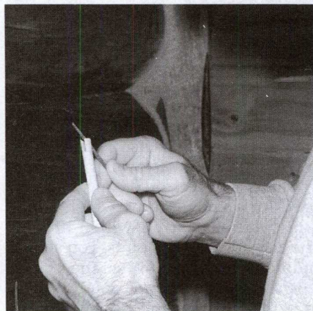
Arrow nocks are made by sawing a slot in the shaft and then enlarging it with a small rattail file. Final work on the nocks will be done with fine sandpaper.
