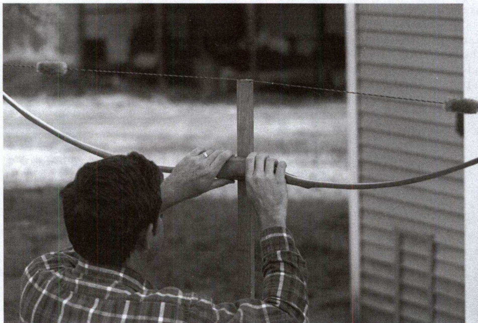
Placing the bowstring in the groove on top of the weighing stick.
