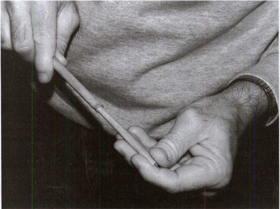
The foreshaft of a river cane arrow should be made of hardwood and fitted into the pile end. The joint will later be wrapped securely with sinew.
