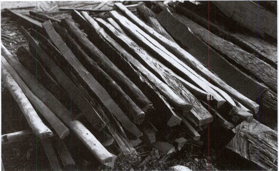
A stack of bandsawn staves, arranged so that air can circulate between them.
