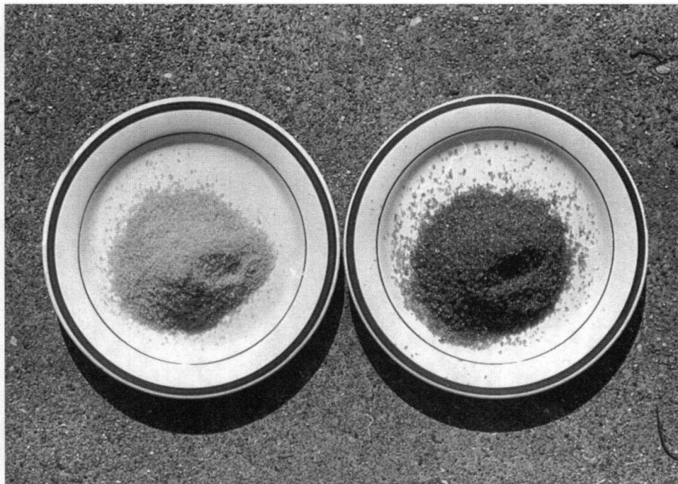
Two commercial "hide" glues. As a general rule, lighter colored glues (left) are stronger. Darker glues are likely bone glues. Stronger glues also smell "cleaner", while weaker ones have a sweet, oily smell, especially when hot and wet.
