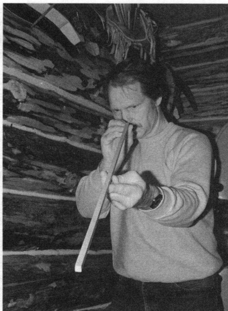
Check to see that all sides of the square dowel are straight and true.
