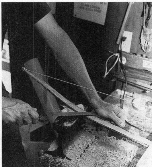
Rasping wood from the belly of a strung bow held in a vice.
