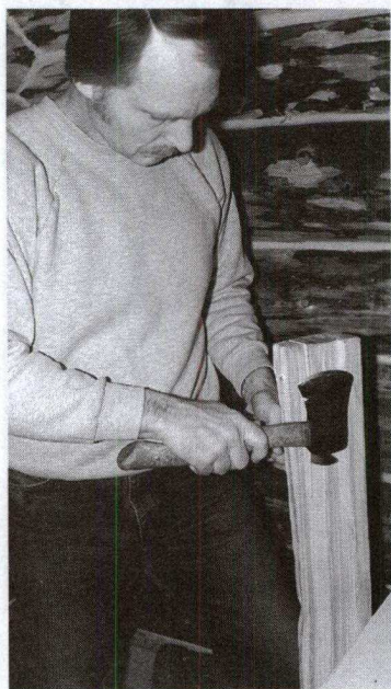
Splitting out an arrow blank is easy with straight-grained wood such as Sitka spruce.
