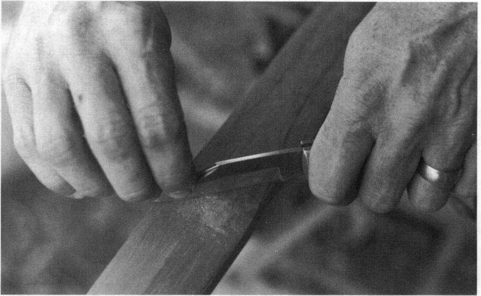
The extra wood around knots is reduced and made symmetrical with a scraper, such as a pocketknife.
