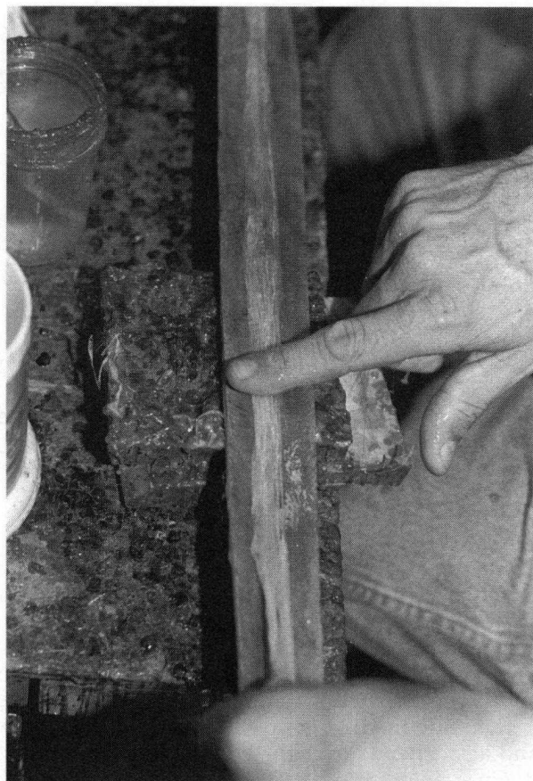
Laying first row of sinew down the center of the bow.
