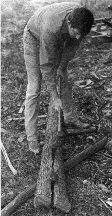
Using a sledgehammer and wedges to split half of a small Osage log.
