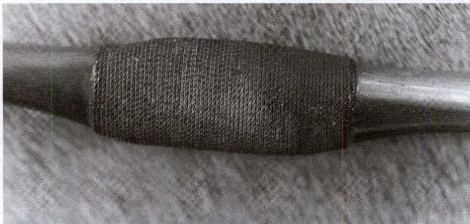
Sixty-year-old bow with braided fishing line wrapped around the handle, then varnished. This makes a simple, effective, and attractive grip. (courtesy Glenn Parker).
