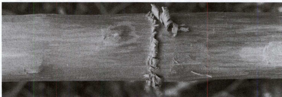
Back of a stave as it appears while drawkniving. Single ring has been established for back at left. Note "islands" of extra wood left around pins.
