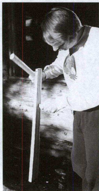
Splitting out an arrow blank is easy with straight-grained wood such as Sitka spruce.
