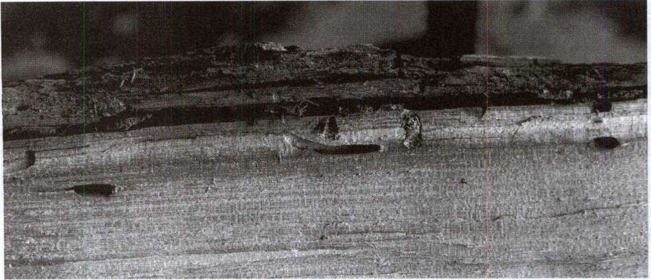
Grub damage in a stave. Note that the holes are all in or near the sapwood.
