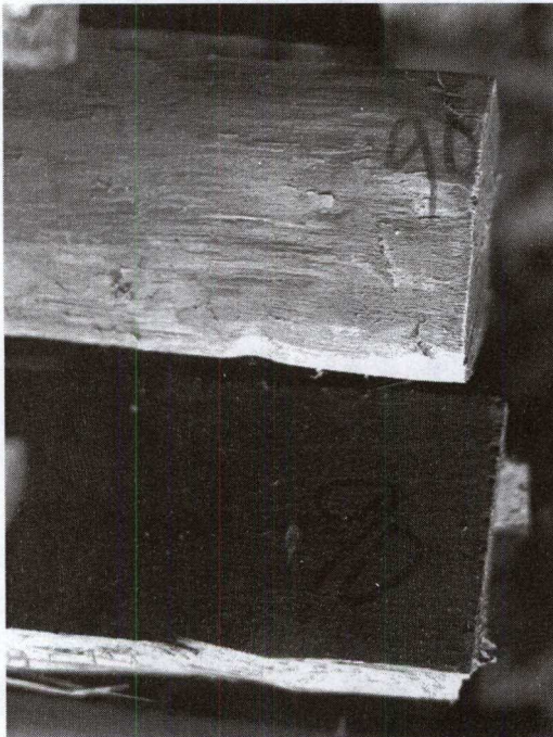
It is a good idea to write a date on each staff, or even a date and the location where the tree was cut, so the drying and the characteristics of the wood can be closely followed.
