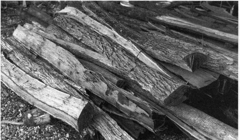
Eight to fifteen inch logs split into quarters to be more easily handled when sawing.
