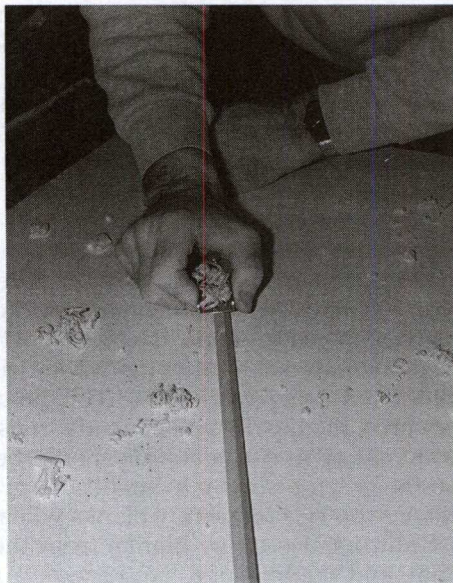
Planing off the four edges of the square dowel gives you an...
