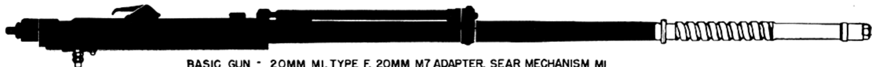
BASIC GUN - 20 MM AN - M2, TYPE E, 20MM AN - MI ADAPTER, ELECTRIC TRIGGER AN - MI, HYDRAULIC CHARGER M1
