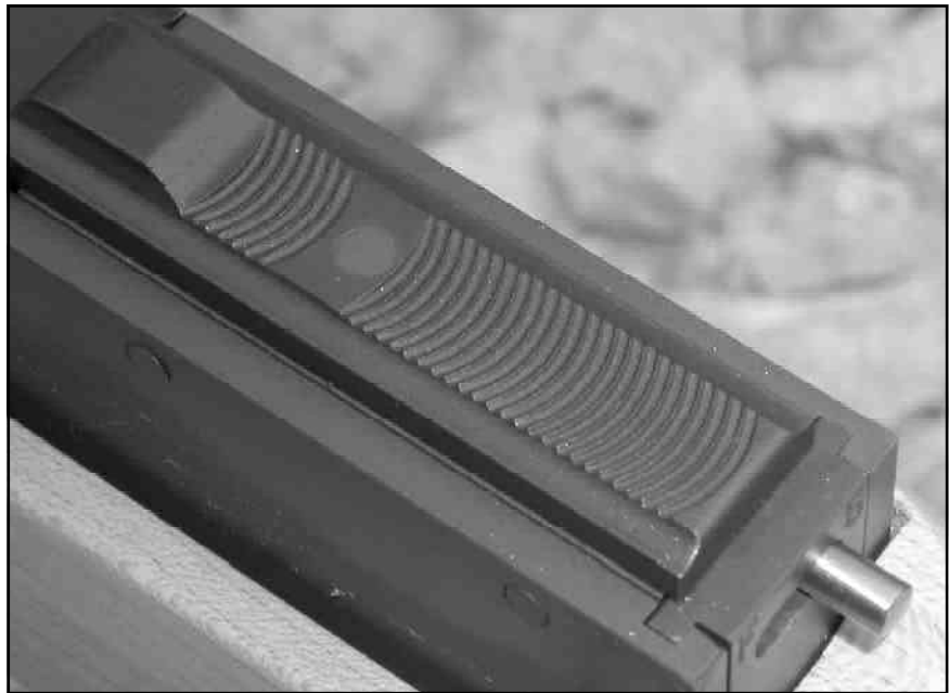
Above: The top cover is different from the rest of the miniature belt-fed firearms manufactured by Lakeside Machine. The safety can be seen at the rear of the receiver in the lower right.
