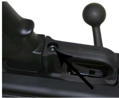
Figure 10 Removing the Grip Frame
