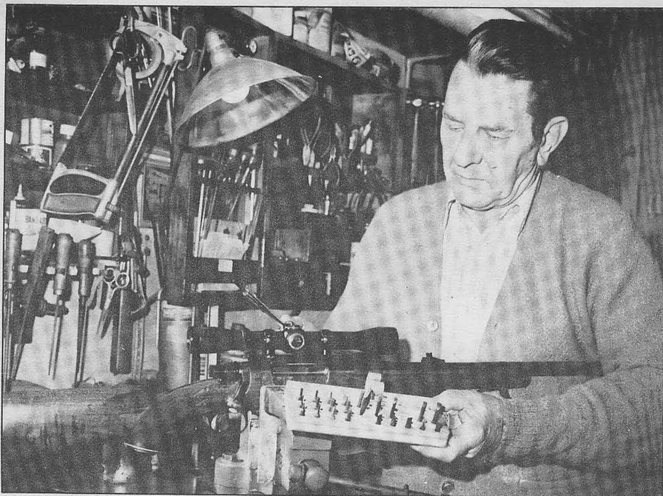
Bish selects the proper size screwdriver from his own collection for use in mounting a rifle scope. He says the proper tools are a necessity for each individual job if one is to achieve status among professional gunsmiths.
