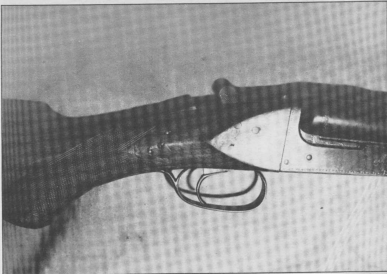
This is another example of what the author considers to be shoddy stock repair work. Nails and brads in the wood only weaken the stock more, while the proper glues or epoxies can strengthen the wood and are unnoticeable.
