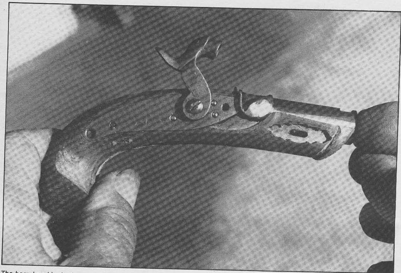
The barrel and lock of the gun must be fitted precisely to the wooden stock, with no gaps, cracks between metal, wood.
