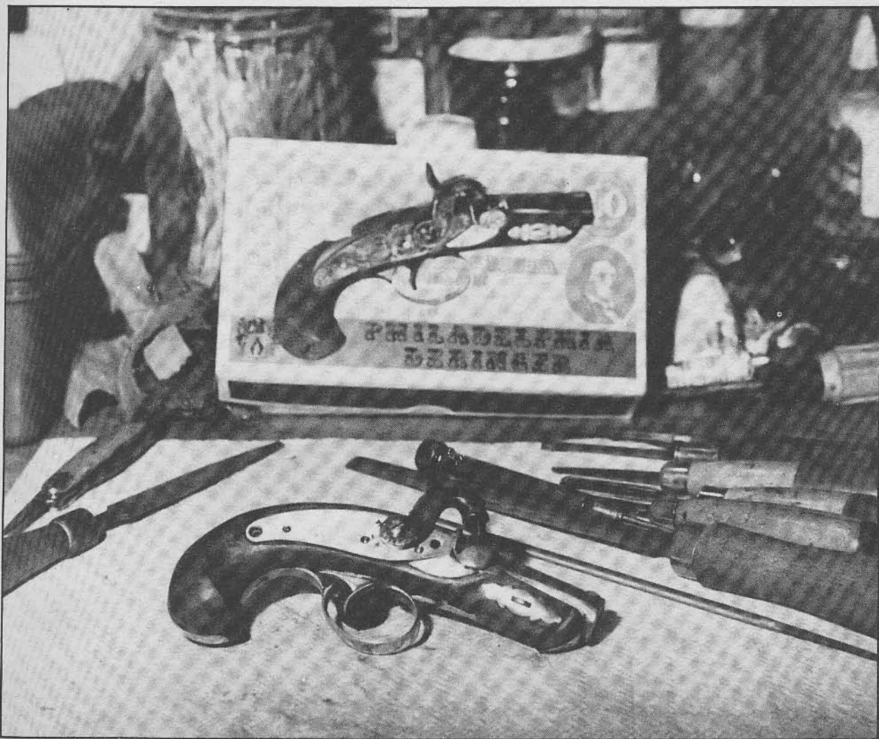
At this point, the derringer is ready for its final finish with Tru-Oil stock finish. However, for the best results, the finish should be used only sparingly, with craftsman sanding the wood lightly between application of the coats.
