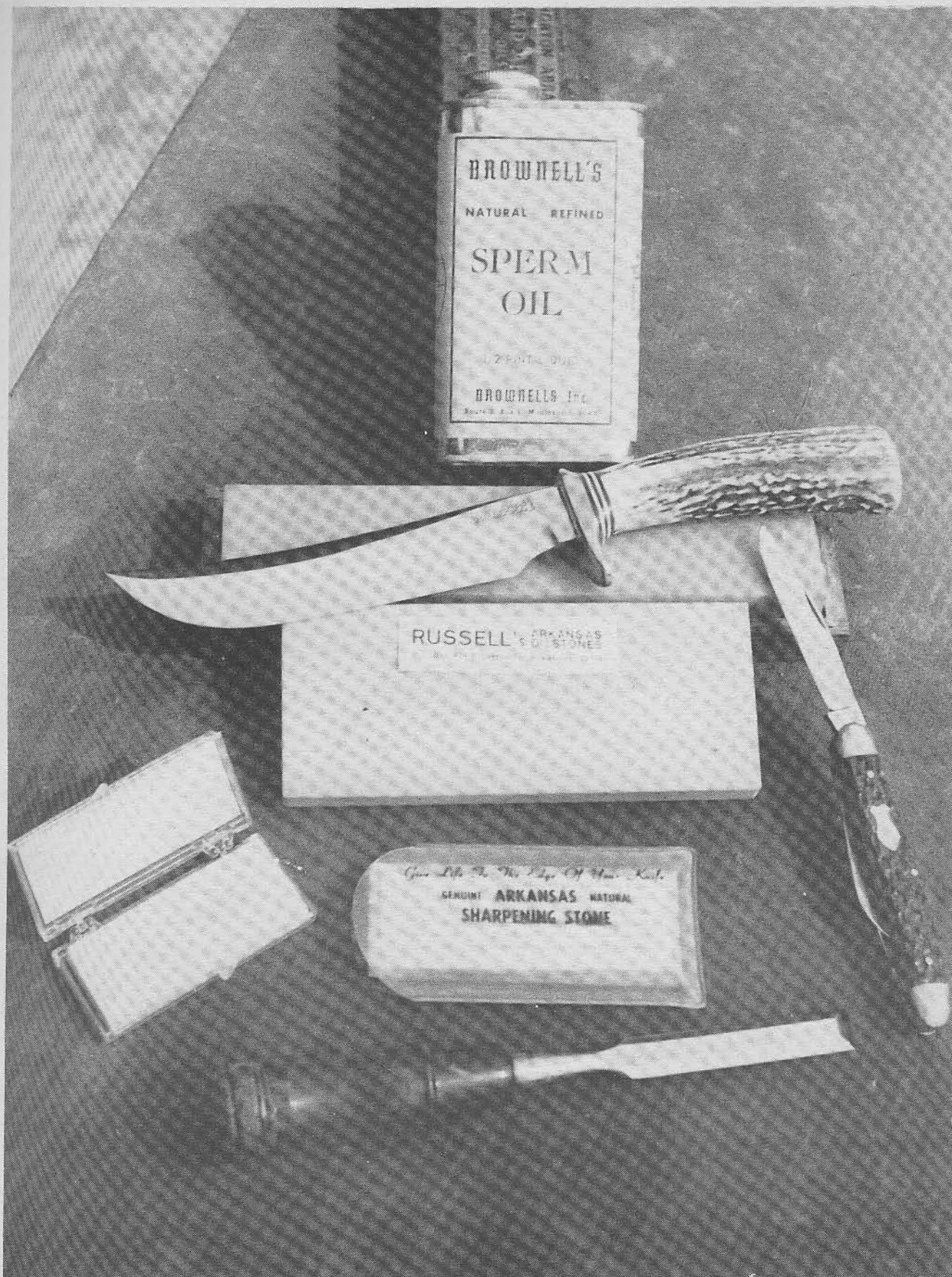
Necessities for maintaining an edge on any cutting tool should include an array of good oil stones and a can of honing oil, although even saliva can be used in lieu of oil in an emergency. There are numerous manufacturers.
