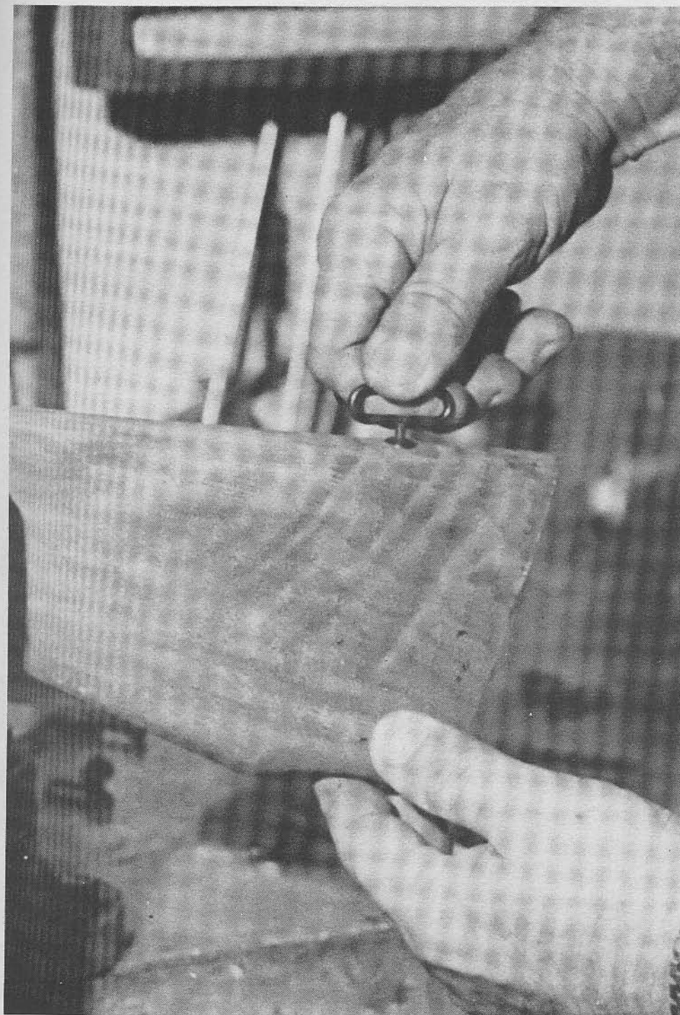
With previous steps completed, the swivel then is inserted, turned to the lock position.
