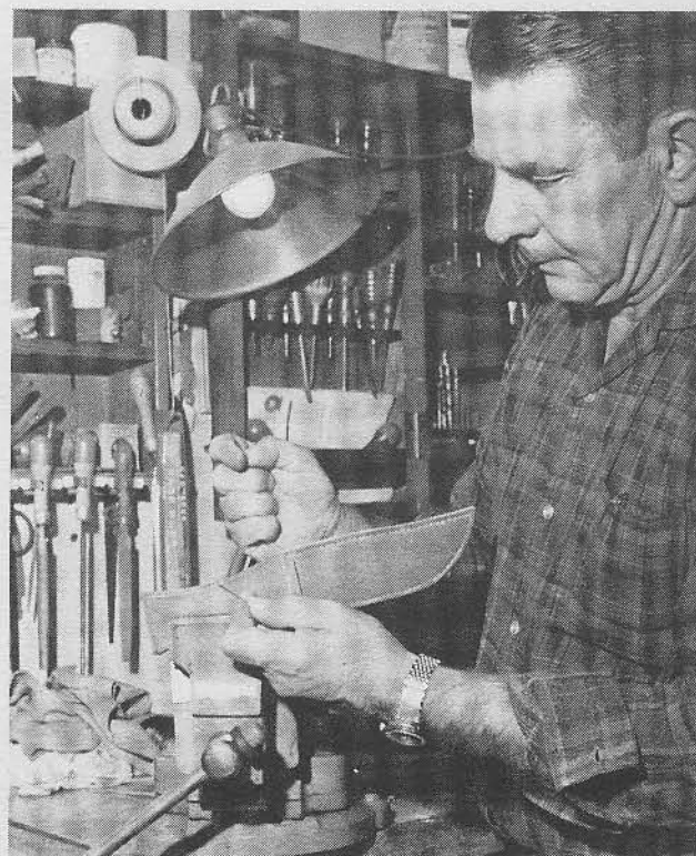
Saddlemakers' stitch calls for passing each needle through same hole from opposite side for a lock stitch.
