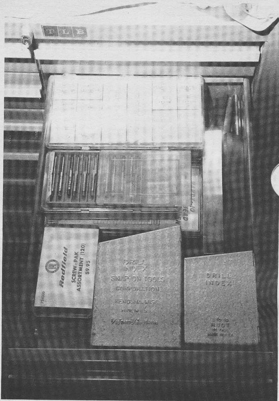
Drawers in your chest should be arranged so related tools are at hand at a moment's notice by opening only one drawer. Drills, taps, assorted dies, as well as sizes of screws are stored in this drawer.
