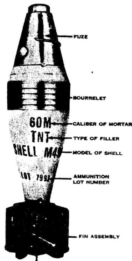
FIGURE 8. SHELL, HIGH EXPLOSIVE M49A2
