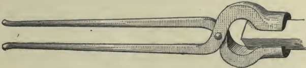
FIG. 98.—TONGS WITH SQUARE, HOLLOW BITS.
