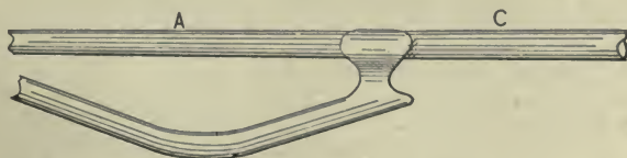
FIG. 153.—SHOWING HOW THE PIECES ARE JOINED AND WELDED IN MAKING AN OFFSET.
