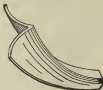
FIG. 170.—SHOWING HOW THE HARROW TOOTH IS BENT.
