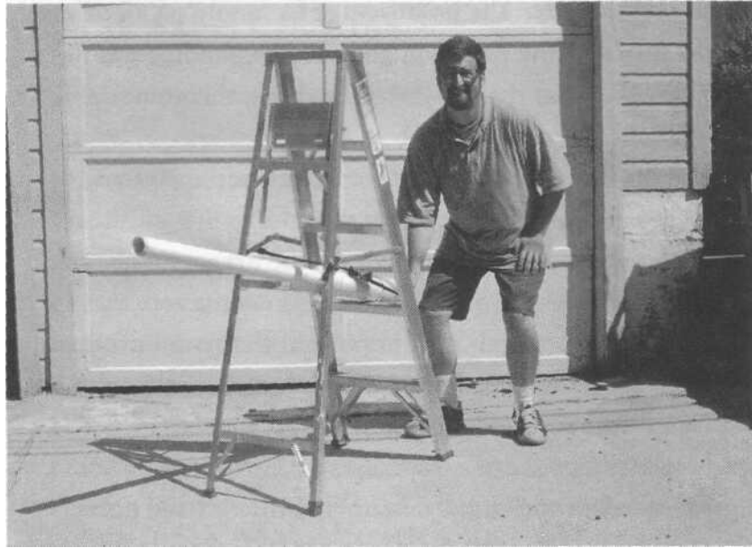
2.7 Using a ladder mount to secure the potato cannon
